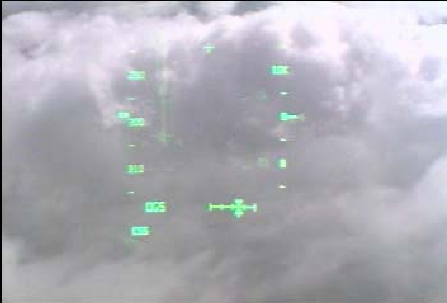
STS 108 Heads Up Display (HUD) on final approach
