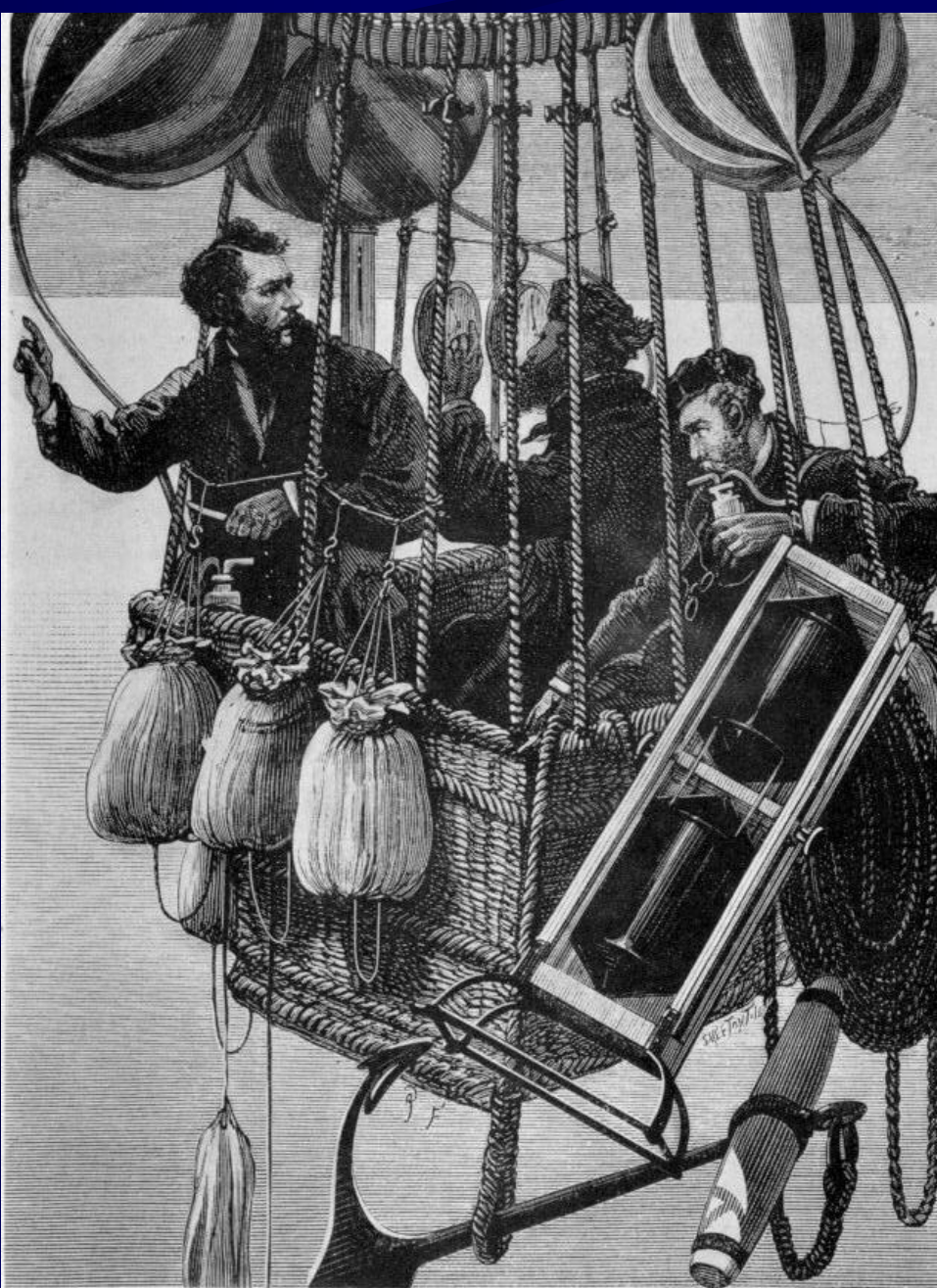
FIG. 2. The famous flight of Tissandier and his two companions, Sivel and Croce-Spinelli in 1875. Sivel is dropping ballast, Tissandier reading the barometer, and Croce-Spinelli is holding his oxygen respirator.
