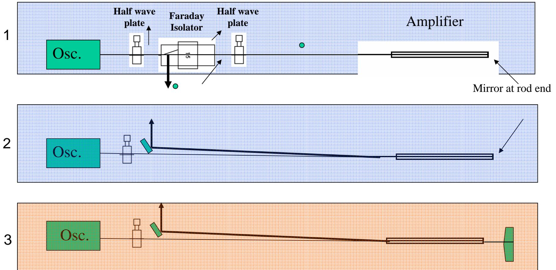
Option 3 selected - Minimum loss, No optical damage, and Optical distortion corrected
