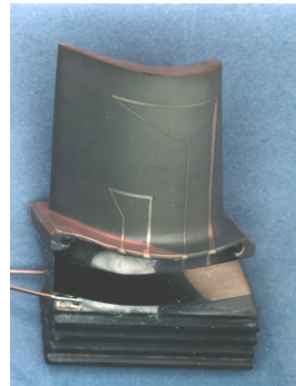
Pt- Pt/Rh temperature sensor to T=1200^{\circ}\text{C}
