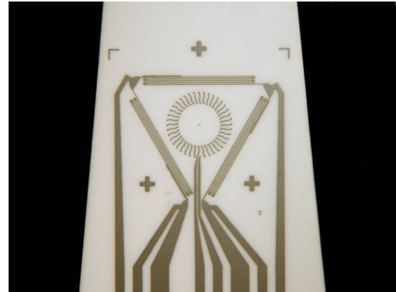
TaN Multifunctional Sensor Strain Output
