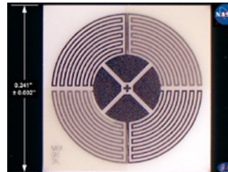
Heat Flux Sensor Array to T=1000^{\circ}\text{C}
