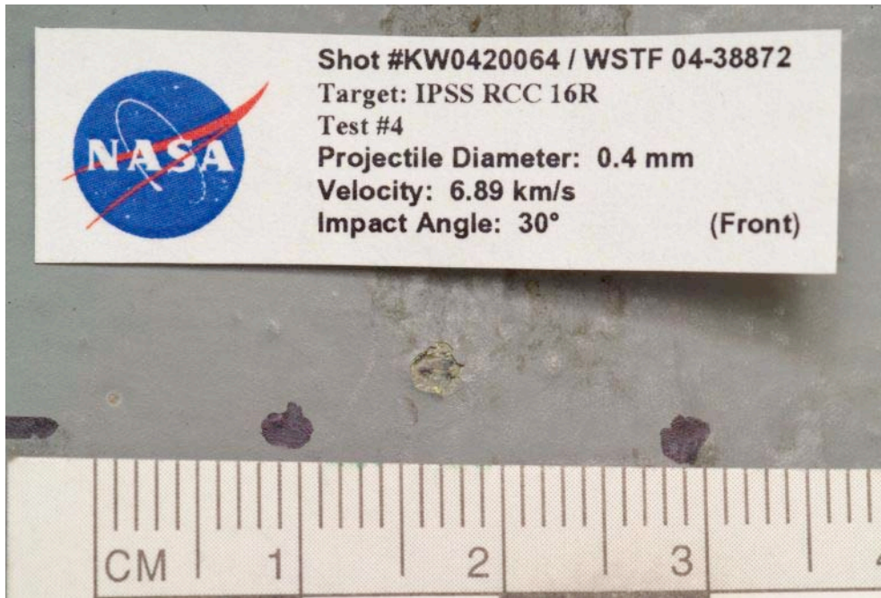
Figure 53: RCC16R Shot #4 Impact Damage
