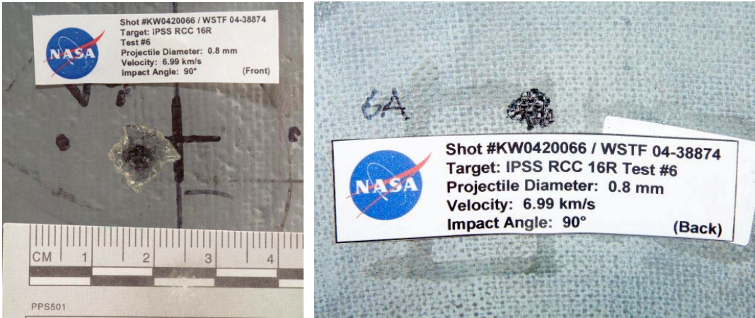
Figure 57: RCC16R Shot #6a Impact Damage (Left: Front Side, Right: Back Side)
