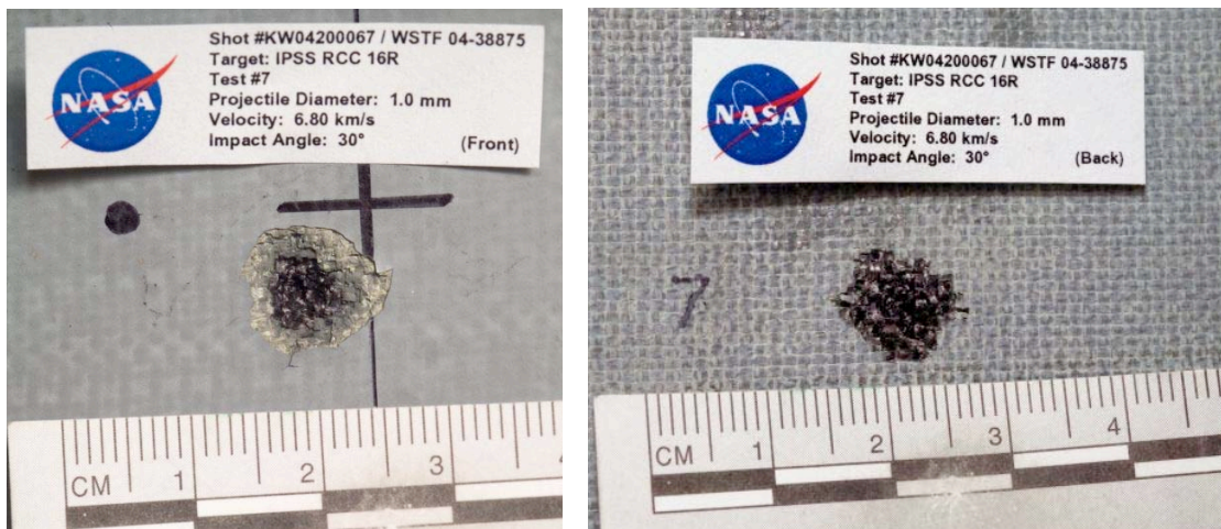
Figure 59: RCC16R Shot #7 Impact Damage (Left: Front Side, Right: Back Side)
