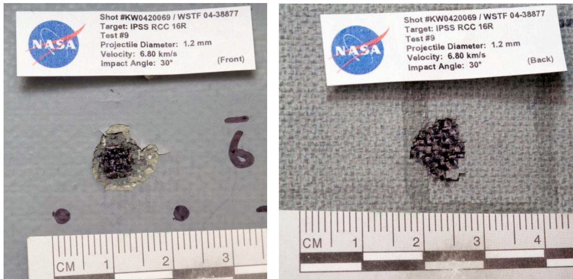
Figure 63: RCC16R Shot #9b Impact Damage (Left: Front Side, Right: Back Side)
