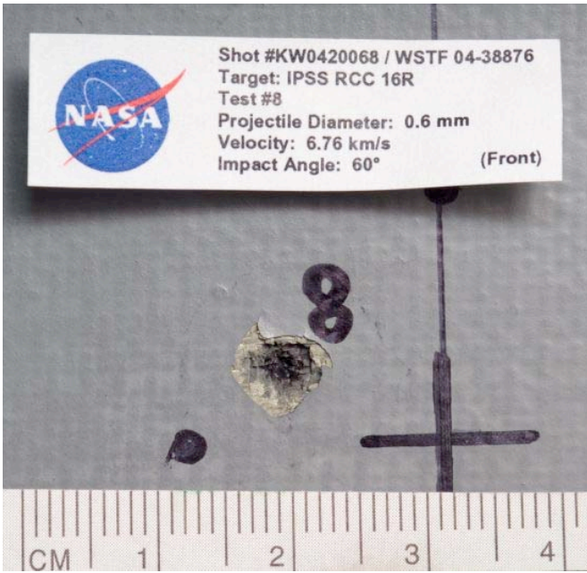
Figure 61: RCC16R Shot #8 Impact Damage
