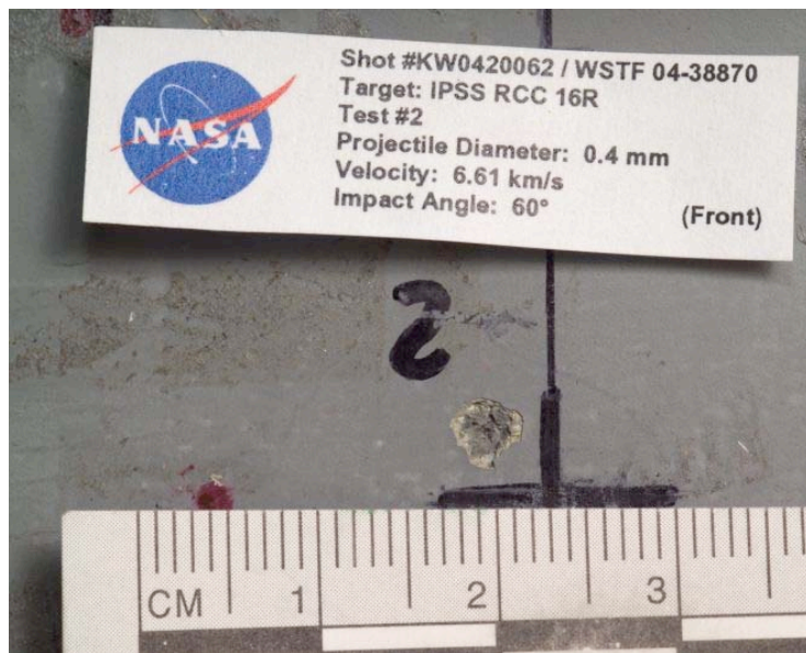
Figure 49: RCC16R Shot #2 Impact Damage
