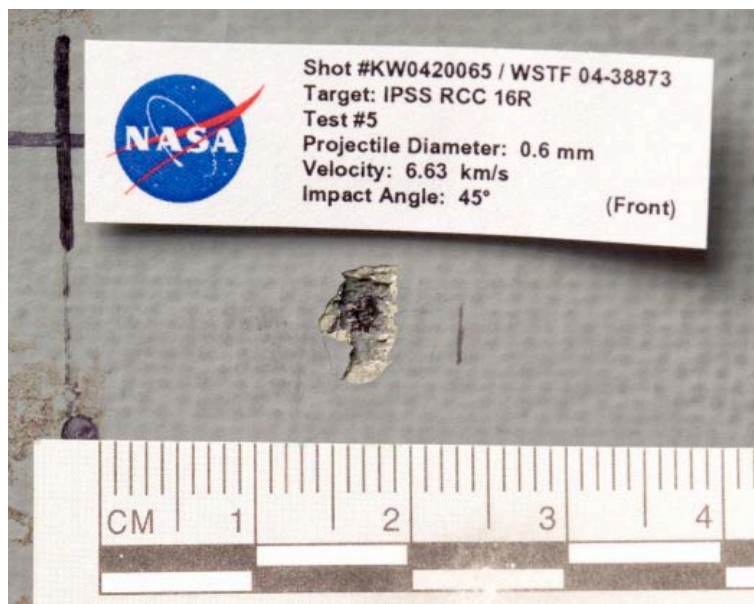
Figure 55: RCC16R Shot #5 Impact Damage
