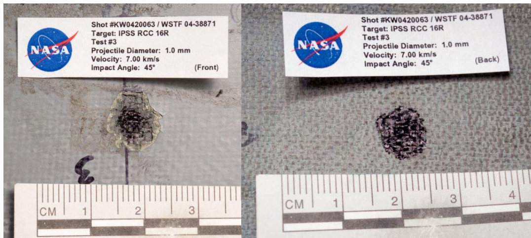
Figure 51: RCC16R Shot #3 Impact Damage (Left: Front Side, Right: Back Side)
