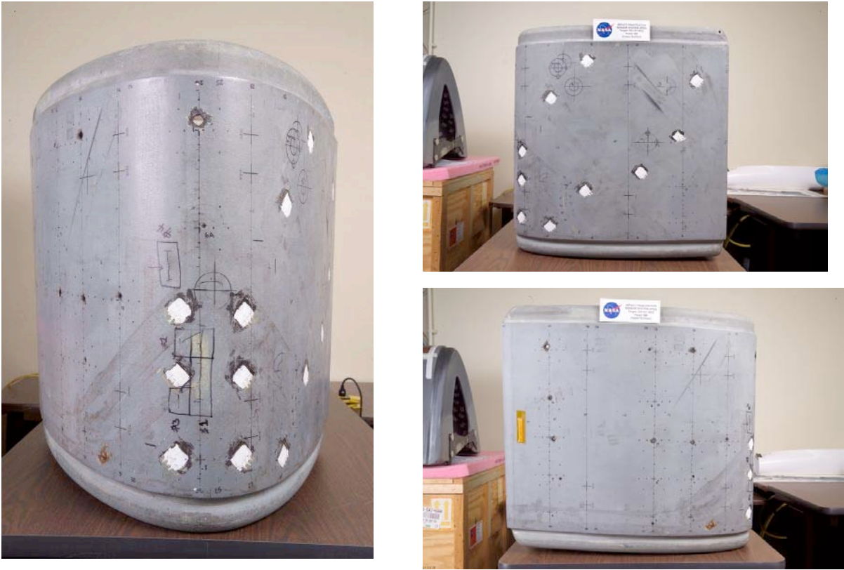
Figure 9: RCC16R Post-test Impact Locations. Left: Front View. Upper Right: Right View. Lower Right: Left View.
