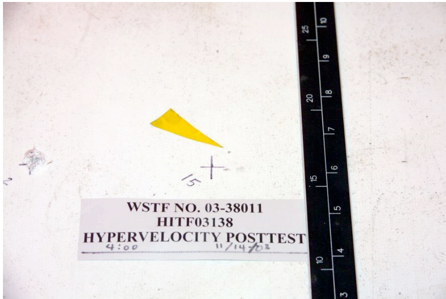
Figure 62: A-2 Shot #15 Impact Damage
