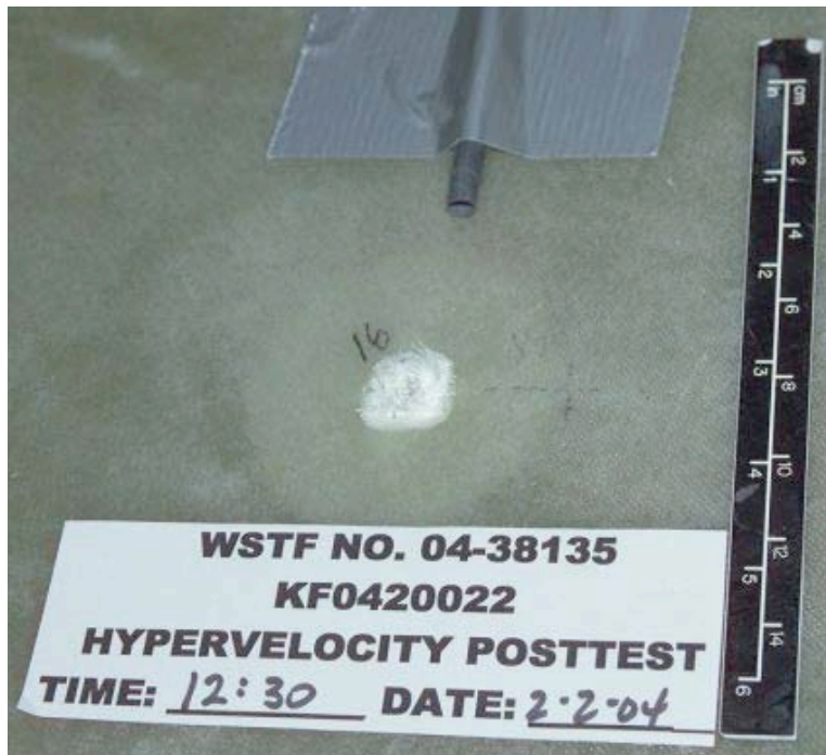
Figure 53: C-1 Shot #16 Impact Damage
