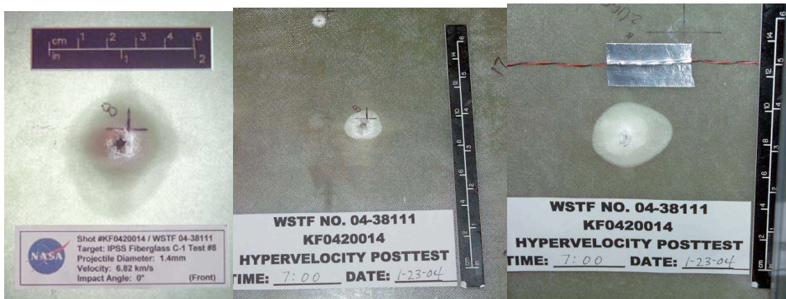
Figure 38: C-1 Shot #8 Impact Damage (Left: Back Illuminated, Middle: Front View, Right: Back View)
