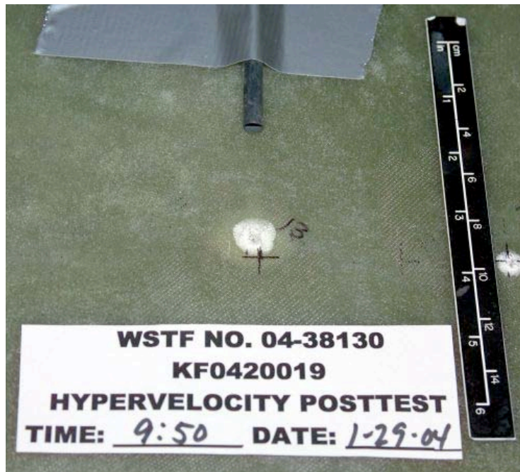
Figure 48: C-1 Shot #13 Impact Damage
