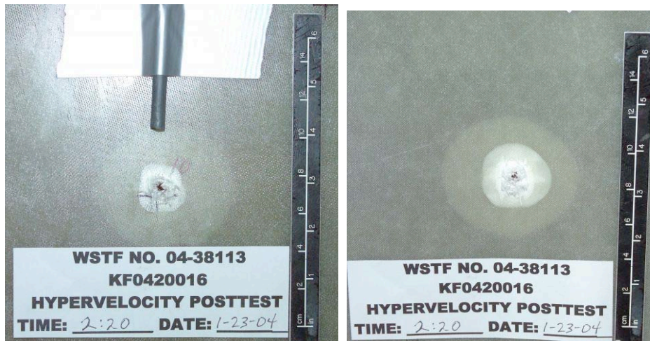
Figure 42: C-1 Shot #10 Impact Damage (Left: Front View, Right: Back View)
