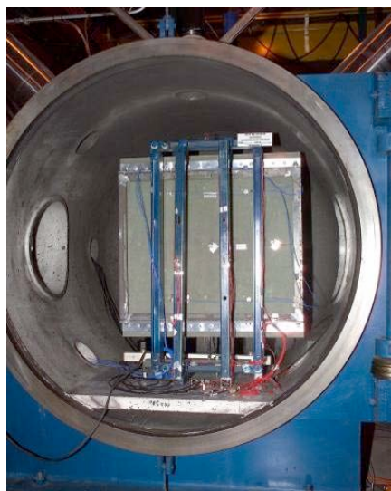
Figure 2: Fiberglass Panel Target C-2 with 90 deg Impact Angle. Back Side View.
