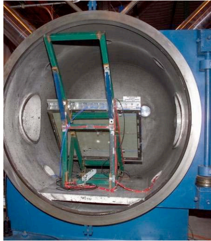
Figure 3: Fiberglass Panel Target C-2 with 45 deg Impact Angle. Back side View.
