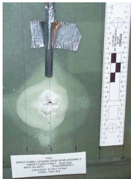
Figure 139: Fg(RCC)-1 Shot #29 Impact Damage
