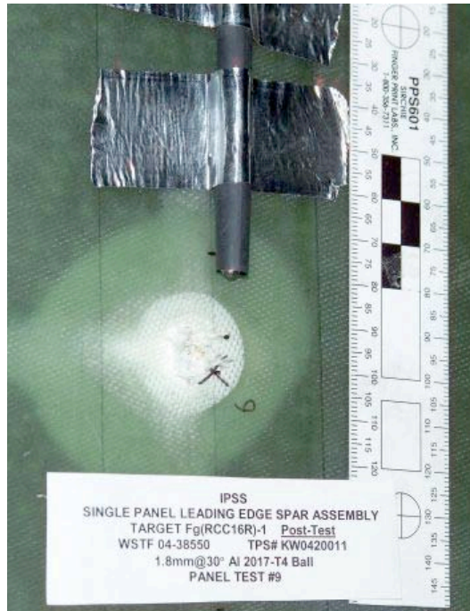
Figure 76: Fg(RCC)-1 Shot #9 Impact Damage
