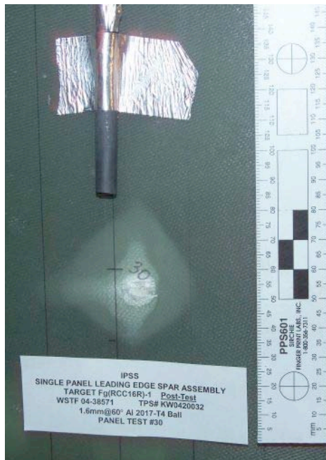
Figure 142: Fg(RCC)-1 Shot #30 Impact Damage
