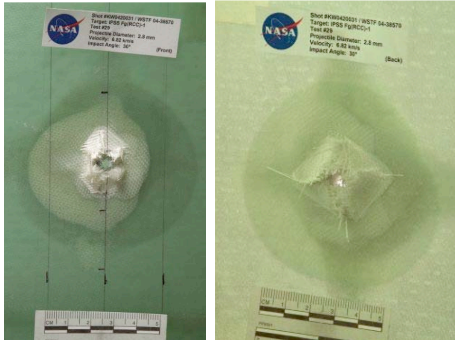
Figure 140: Fg(RCC)-1 Shot #29 Backlit Impact Damage (Left: Front Side, Right: Back Side)
