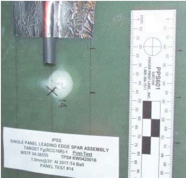
Figure 91: Fg(RCC)-1 Shot #14 Impact Damage
