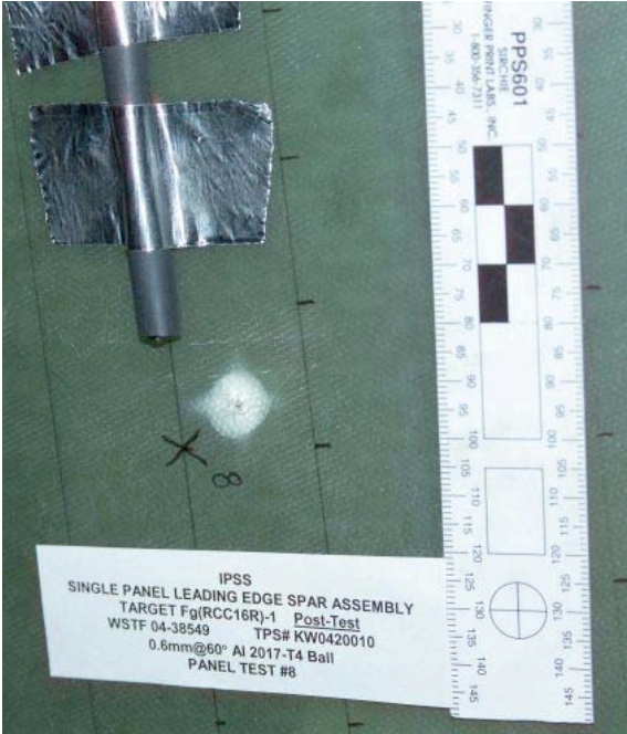
Figure 73: Fg(RCC)-1 Shot #8 Impact Damage
