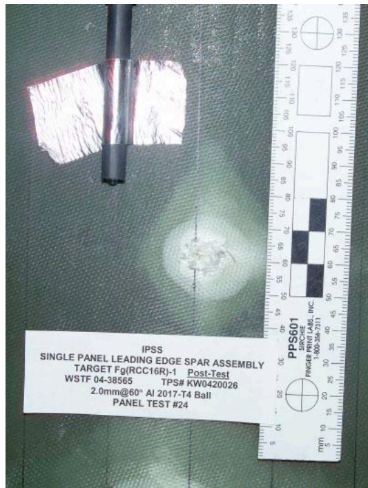
Figure 124: Fg(RCC)-1 Shot #24 Impact Damage
