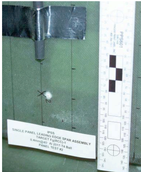
Figure 55: Fg(RCC)-1 Shot #2 Impact Damage
