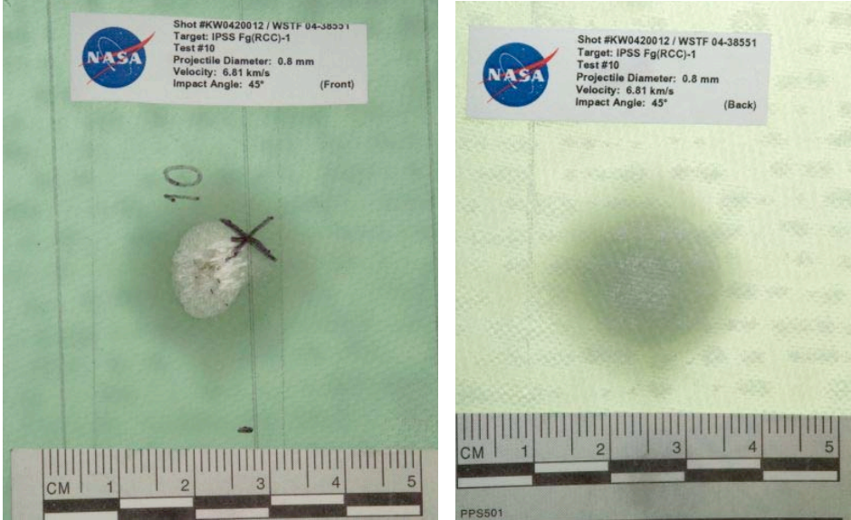
Figure 80: Fg(RCC)-1 Shot #10 Backlit Impact Damage (Left: Front Side, Right: Back Side)
