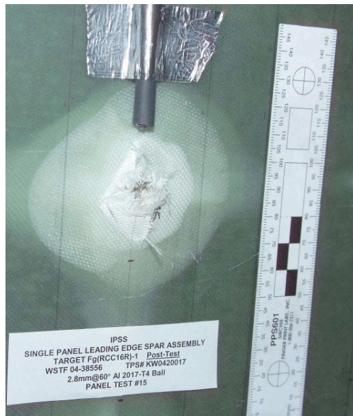
Figure 94: Fg(RCC)-1 Shot #15 Impact Damage
