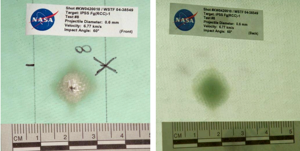
Figure 74: Fg(RCC)-1 Shot #8 Backlit Impact Damage (Left: Front Side, Right: Back Side)
