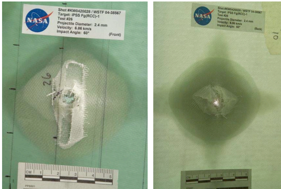
Figure 131: Fg(RCC)-1 Shot #26 Backlit Impact Damage (Left: Front Side, Right: Back Side)
