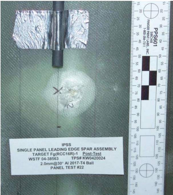
Figure 118: Fg(RCC)-1 Shot #22 Impact Damage
