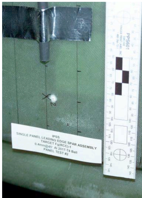
Figure 58: Fg(RCC)-1 Shot #3 Impact Damage
