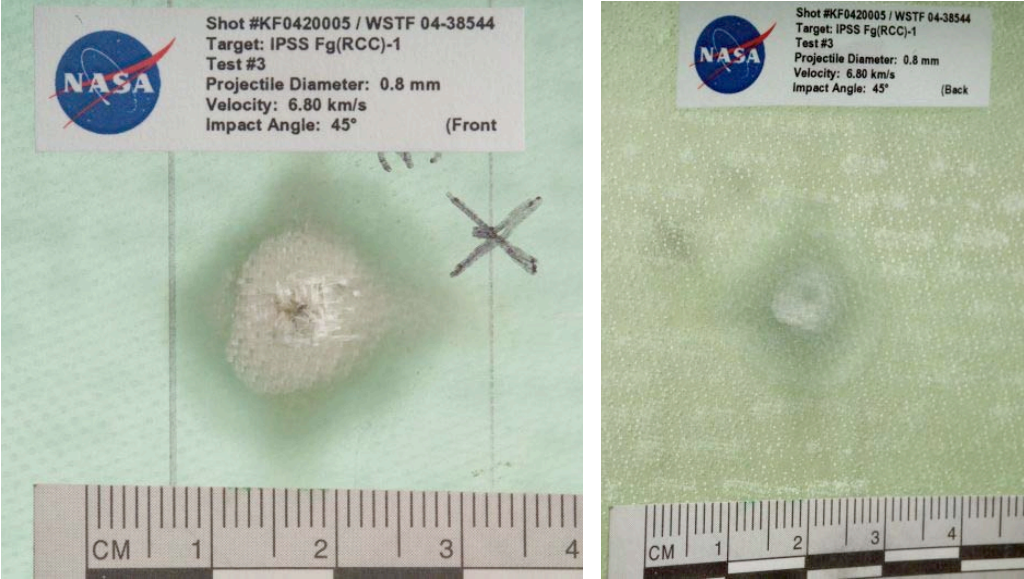
Figure 59: Fg(RCC)-1 Shot #3 Backlit Impact Damage (Left: Front Side, Right: Back Side)
