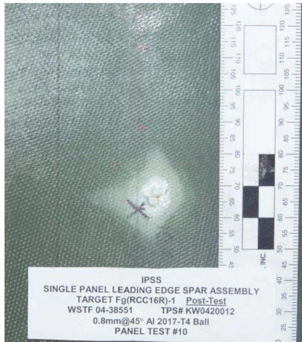
Figure 79: Fg(RCC)-1 Shot #10 Impact Damage
