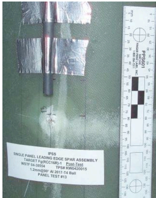
Figure 88: Fg(RCC)-1 Shot #13 Impact Damage
