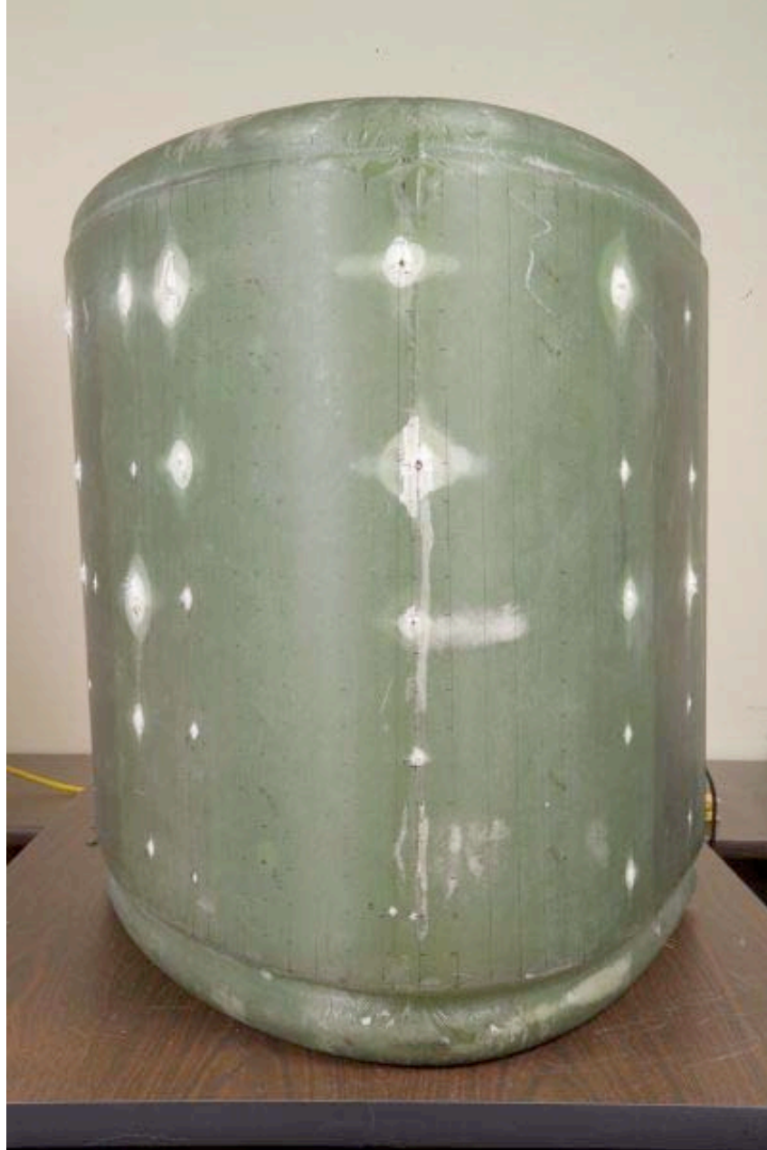
Figure 9: Fg(RCC)-1 Post-test Impact Locations. Front View.
