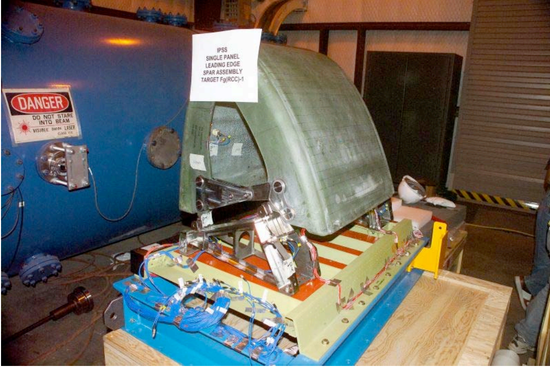
Figure 1: Target Fg(RCC)-1 on Mounting Fixture
