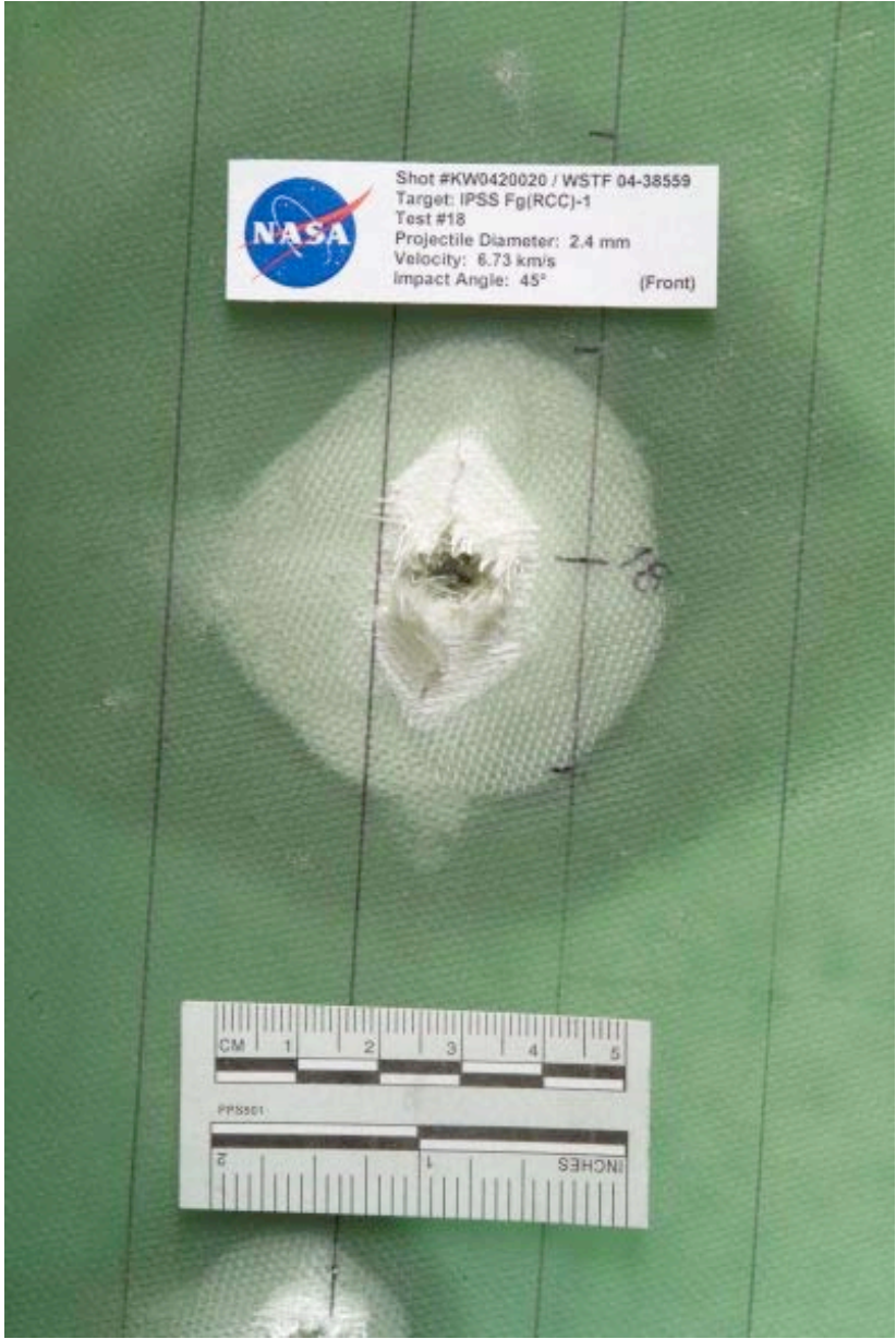
Figure 14: Fg(RCC)-1 Impact Damage Area for Shot #18
