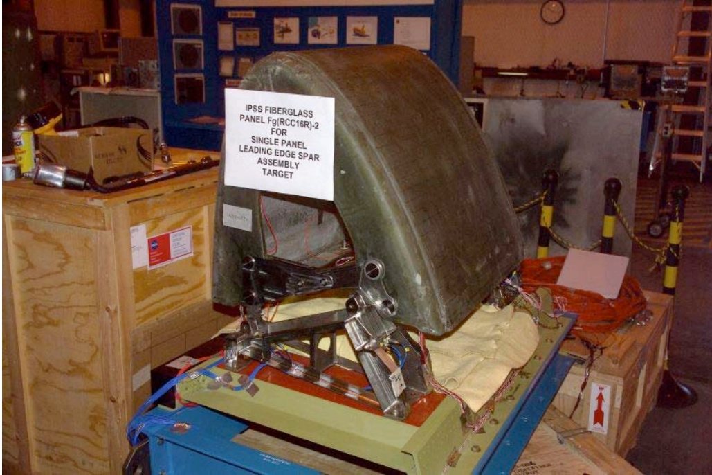
Figure 1: Target Fg(RCC)-2 on Mounting Fixture
