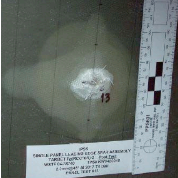
Figure 84: Fg(RCC)-2 Shot #13 Impact Damage
