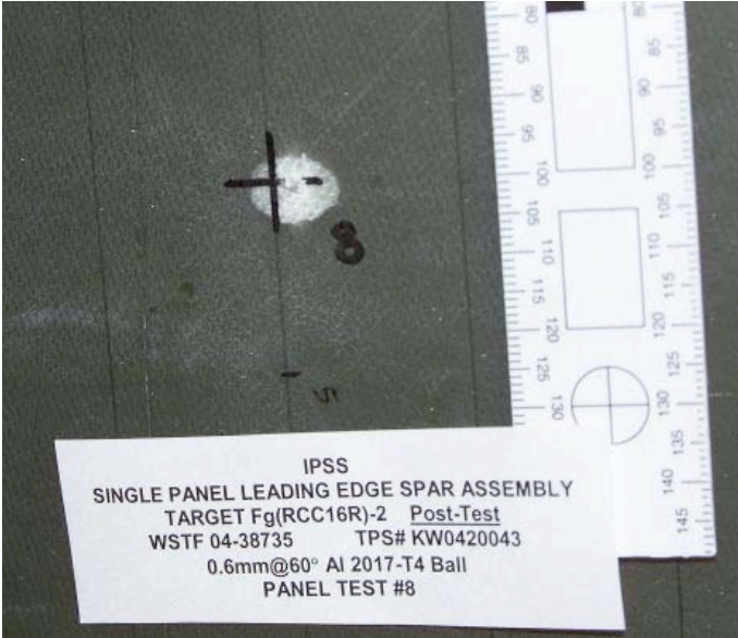
Figure 69: Fg(RCC)-2 Shot #8 Impact Damage
