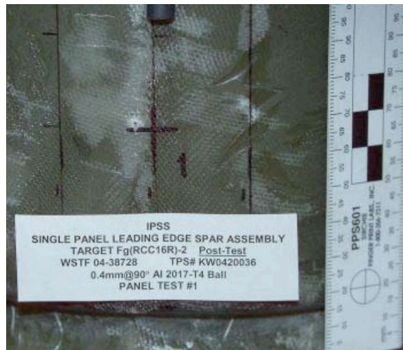
Figure 48: Fg(RCC)-2 Shot #1 Impact Damage
