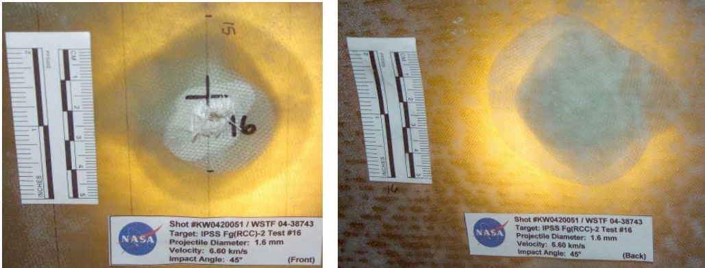
Figure 94: Fg(RCC)-2 Shot #16 Backlit Impact Damage (Left: Front Side, Right: Back Side)
