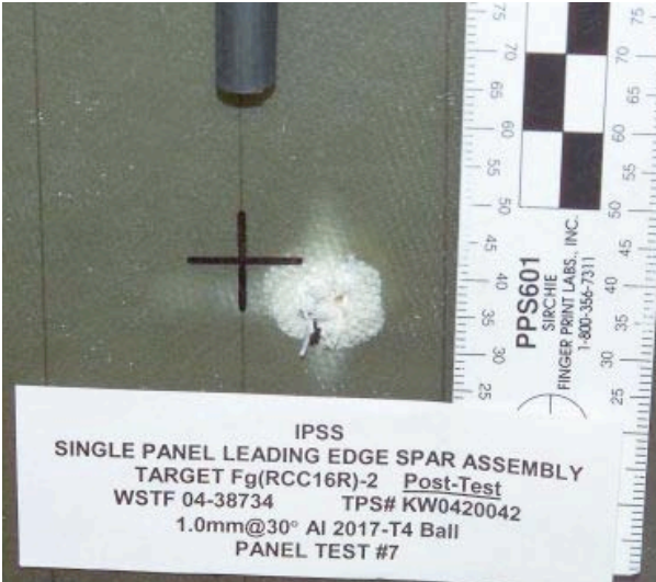
Figure 66: Fg(RCC)-2 Shot #7 Impact Damage
