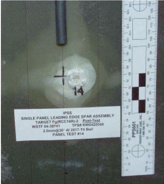
Figure 87: Fg(RCC)-2 Shot #14 Impact Damage
