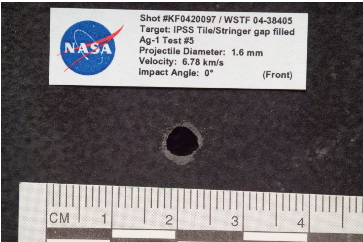
Figure 96: Ag-1 Shot #5 Impact Damage
