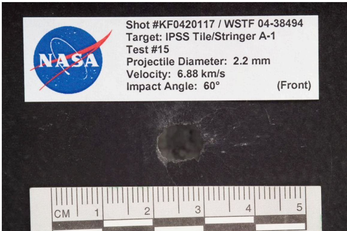
Figure 80: A-1 Shot #15 Impact Damage
