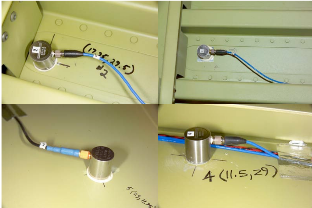
Figure 8: Detail of Acoustic Emission Sensors. Clockwise from Upper Left: Sensor 2 on Target A-1, Sensor 1 on Target Ag-1, Sensor 5 on Target B-1, and Sensor 4 on Target Bg-1
