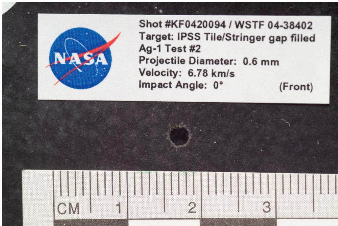
Figure 90: Ag-1 Shot #2 Impact Damage
