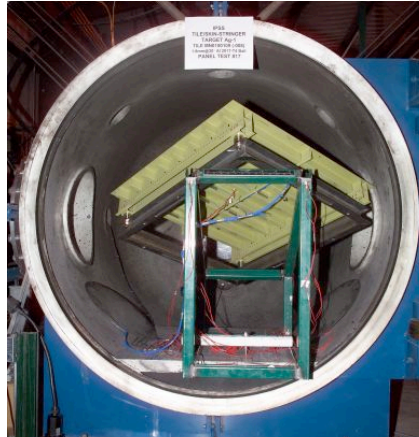
Figure 7: Fiberglass Panel Target Ag-1 with 30 deg Impact Angle. Back Side View.
