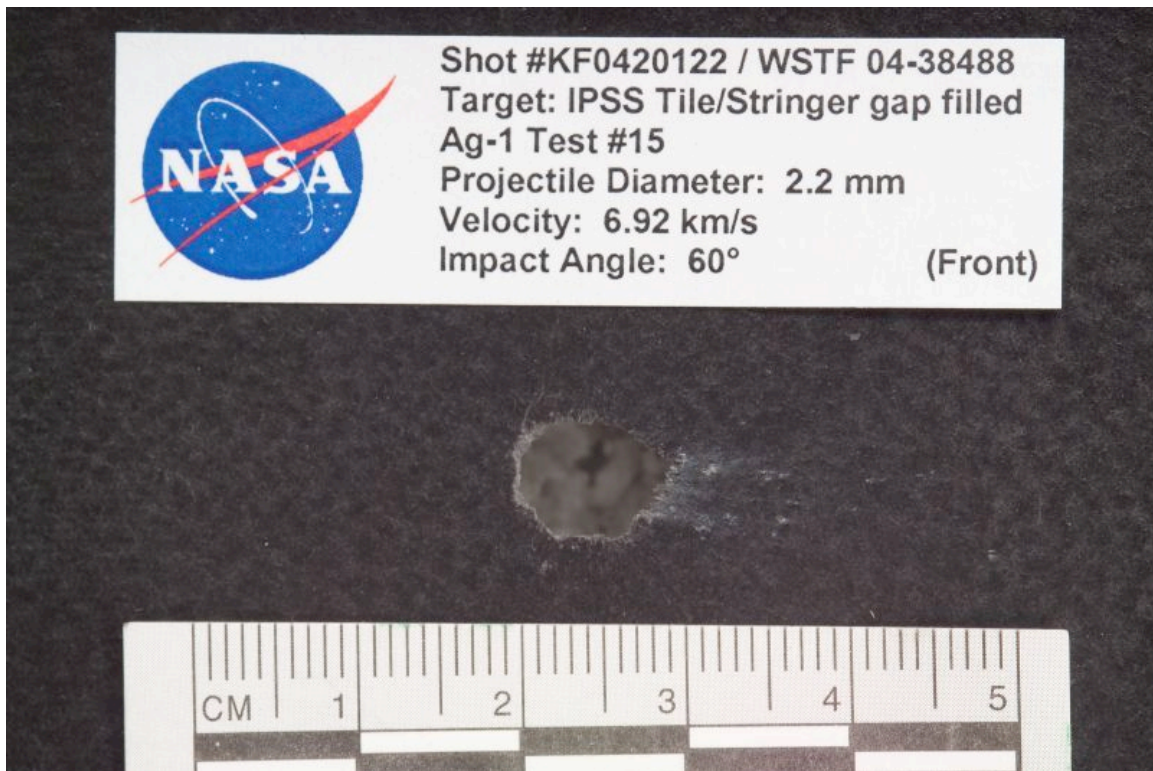
Figure 116: Ag-1 Shot #15 Impact Damage
