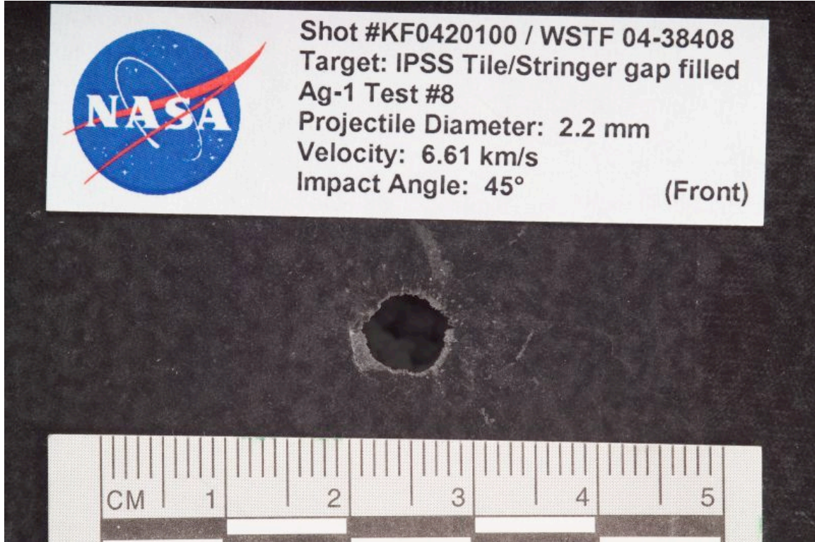
Figure 102: Ag-1 Shot #8 Impact Damage
