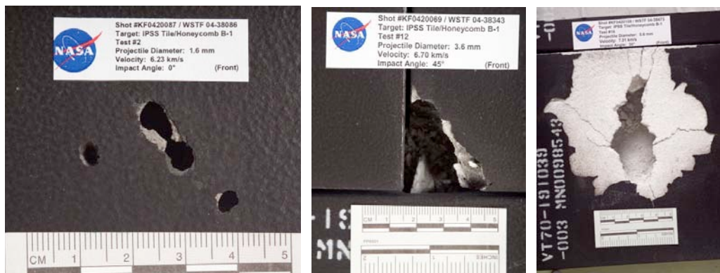
Figure 23: B-1 Impact Damage Area for (Left to Right) Shots #2, 12, and 16
