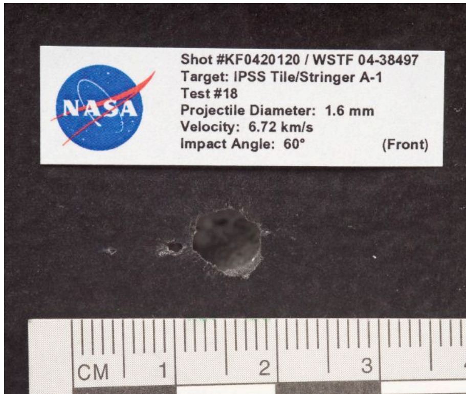
Figure 86: A-1 Shot #18 Impact Damage
