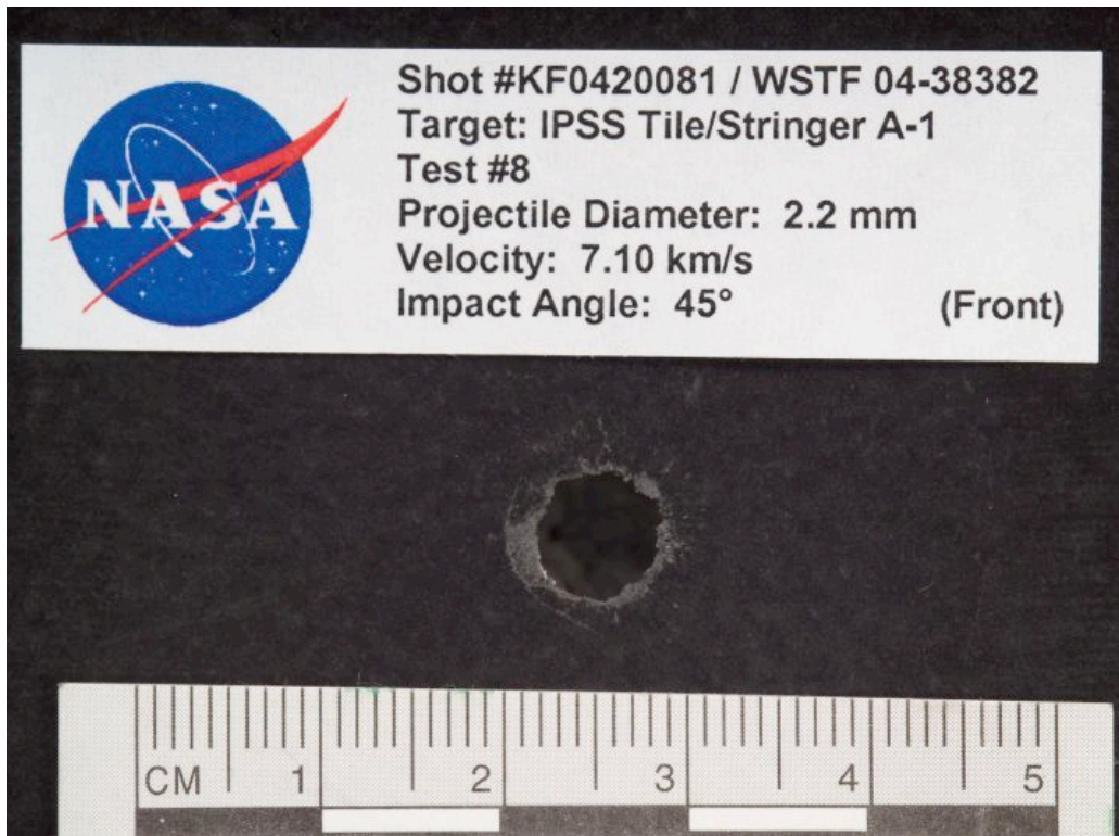
Figure 66: A-1 Shot #8 Impact Damage
