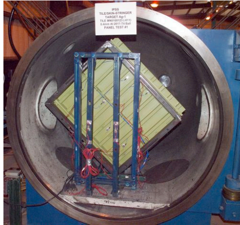
Figure 5: Fiberglass Panel Target Ag-1 with 90 deg Impact Angle. Back Side View.
