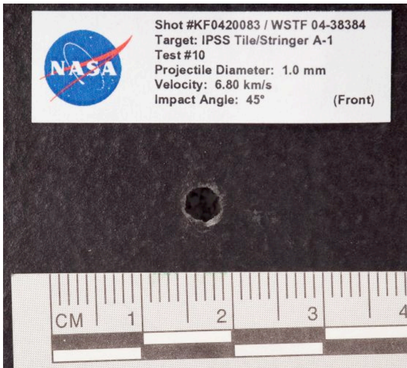
Figure 70: A-1 Shot #10 Impact Damage
