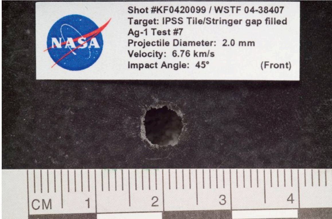
Figure 100: Ag-1 Shot #7 Impact Damage
