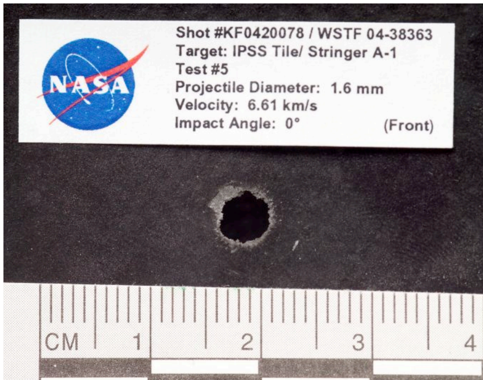
Figure 60: A-1 Shot #5 Impact Damage
