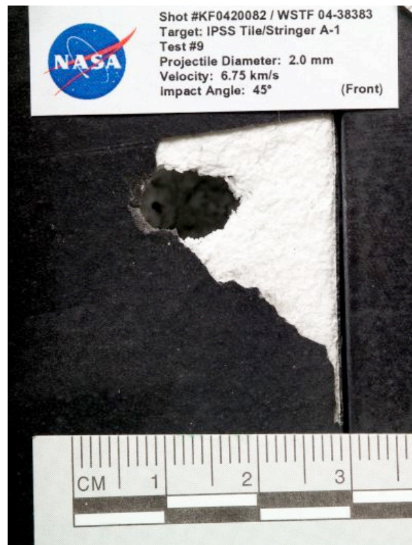
Figure 68: A-1 Shot #9 Impact Damage
