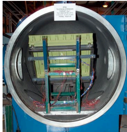
Figure 6: Fiberglass Panel Target Ag-1 with 45 deg Impact Angle. Back Side View.
