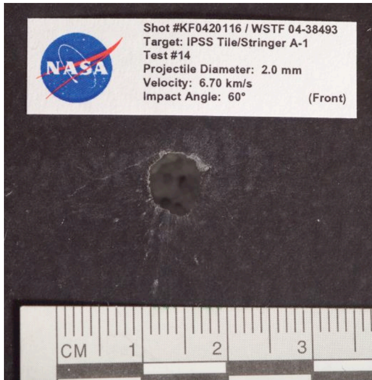
Figure 78: A-1 Shot #14 Impact Damage
