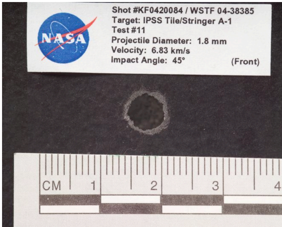
Figure 72: A-1 Shot #11 Impact Damage
