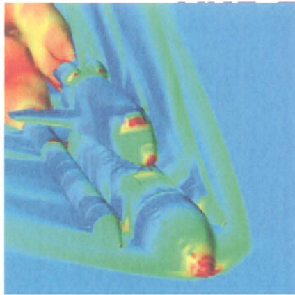
Figure 1. Pressure Coefficient on the Space Shuttle Launch Vehicle and in the Near-Body Flowfield [4]
