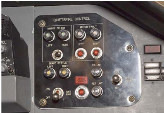
Figure 6. Quiet Spike control panel in the rear cockpit.
