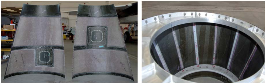
Figure 9. Quiet Spike nose cone modifications.
