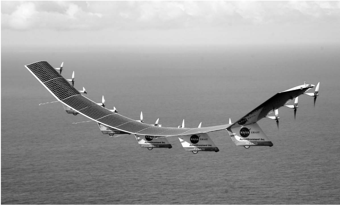
Figure 1. Solar powered Helios prototype flying wing during a test flight over the Pacific Ocean.
