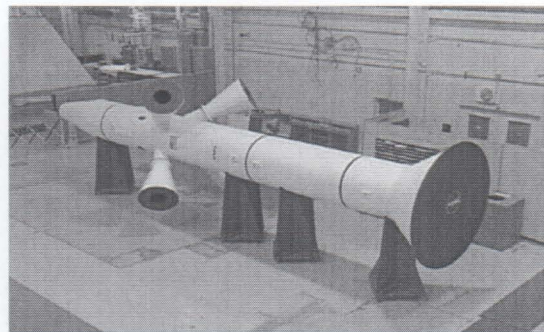
Figure 9. Launch Abort System (LAS) mockup on Langley Research Center shop floor for servicing access testing.
