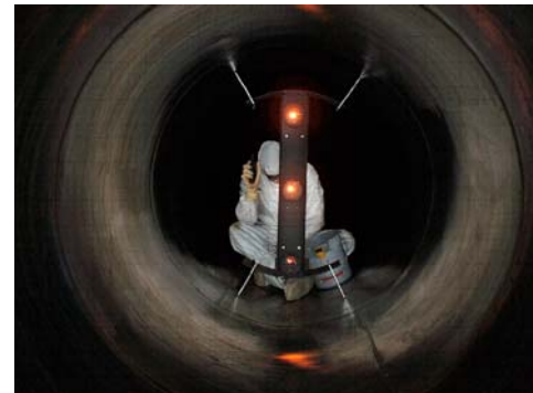
Figure 11. DART target during 500 meter vacuum tunnel testing
