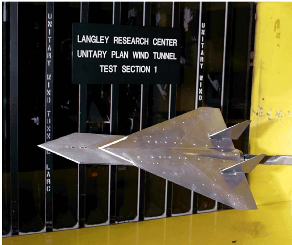
Figure 1. Photograph of the porous LEX model installed in Test Section 1 of the NASA Langley Research Center Unitary Plan Wind Tunnel.
