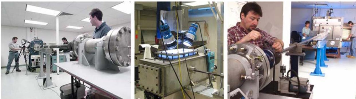
Figure 5.—From left to right; small vacuum chamber, particle gun chamber, and large vacuum chamber guns at the NASA Glenn Ballistic Impact Facility.
