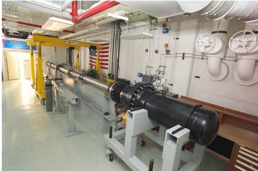
Figure 6.—Eight inch gun at the NASA Glenn Ballistic Impact Facility.
