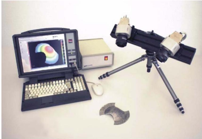
Figure 8.—Aramis 3D deformation/strain measurement system shown with static camera assembly.
