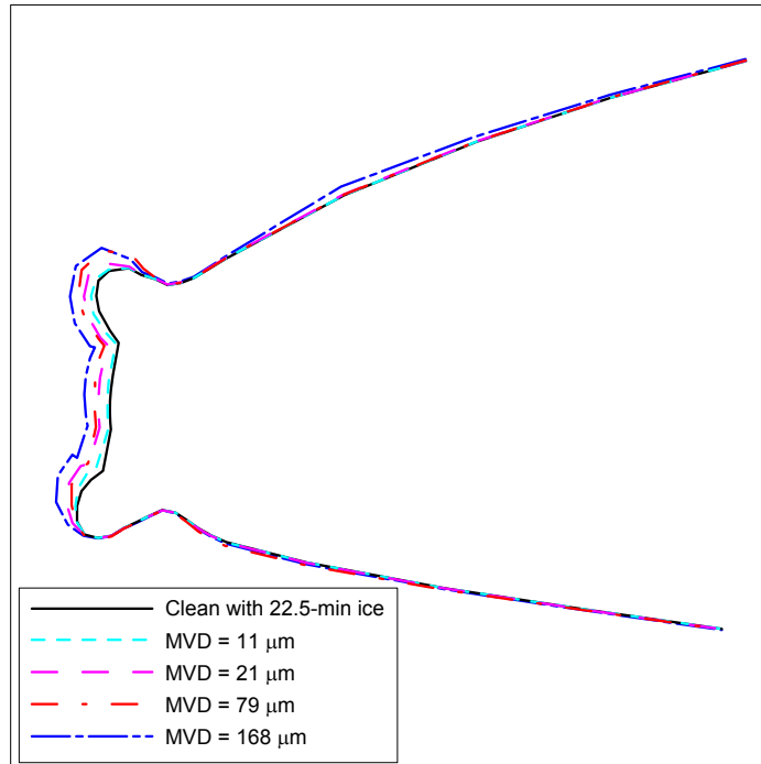
Figure 109.—Experimental impingement efficiency surface distribution for Twin Otter tail with 22.5-min ice shape at AOA=0°.
