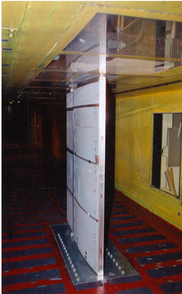
Figure 32c.—Twin Otter tail with 22.5-min ice shape installed in IRT test section.
