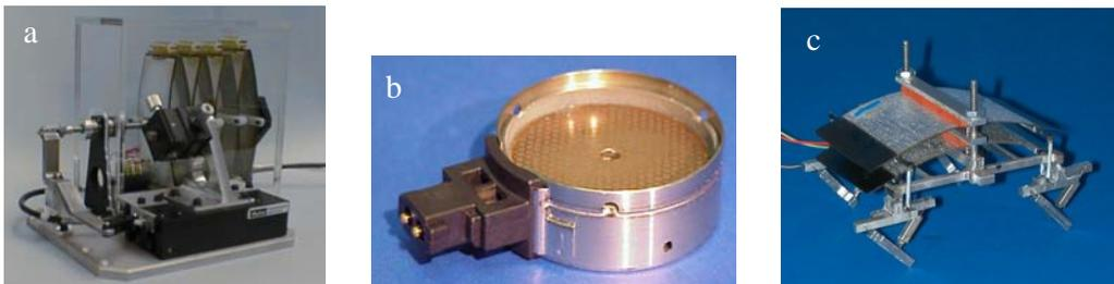
Figure 9. (a) THUNDER linear spectrometer motor, (b) Diesel valve injector actuator/sensor (c) THUNDER powered robot.
