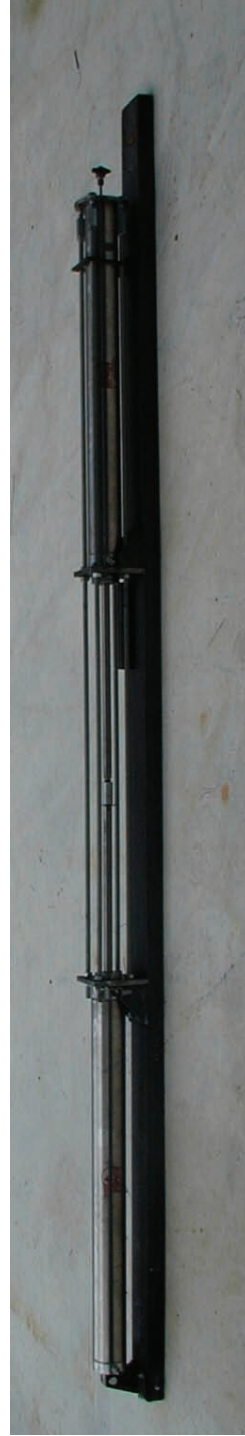
Figure 6. Schematic of PDFB powdered metal feed system and photograph of assembled unit.
