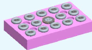
Diagram showing the MISSE 6A and 6B o-ring AO/UV exposure assembly
