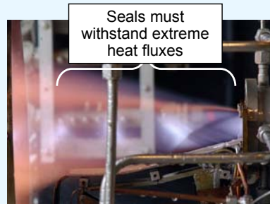
Baseline control surface seal design
