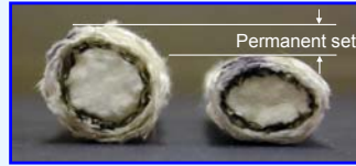
Baseline control surface seal design
