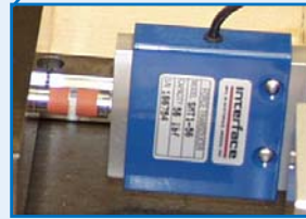
Photograph of an adhesion test in progress showing the deformation before separation (left).
