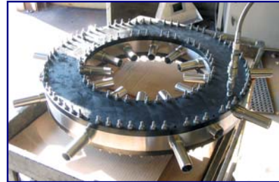
Hydro Test of New Chamber
