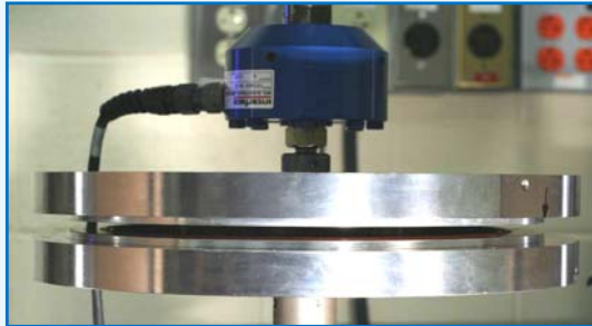
Photo of the compression testing of 12" Gask-o-seals in an axially aligned seal-on-seal configuration.
