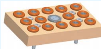
O-ring Exposure Fixture (AO and Non AO sides)
