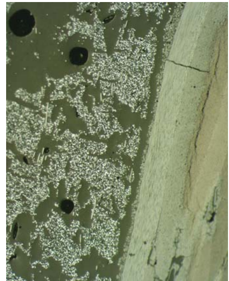
Optical images of GRC 2 at 50 X. The picture (right) shows the interaction of GRABER and the SiC coating. To the left is an image of the gasket material after heating.
