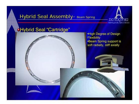
The ATG H-seal utilizes hydrostatic pressures to provide a compliant seal surface. The seal surface is supported by a spring housing that is "soft" radially and stiff axially. The seal utilizes a brush seal as a secondary seal which also provides damping for the hydrostatic bearing surface. The seal components can be modified to handle large radial and axial excursions as well as high temperature and pressure.
