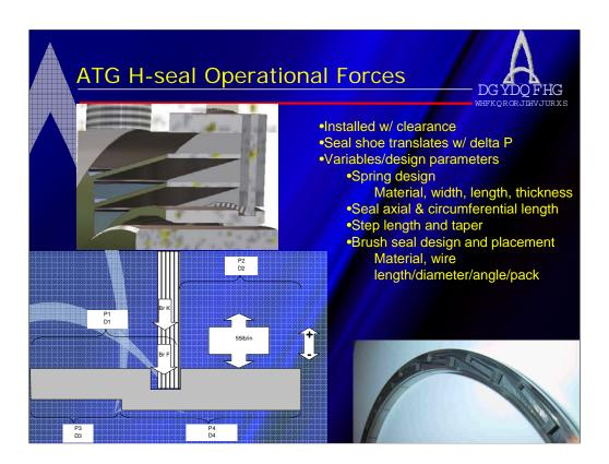
A free body diagram was developed to aid in the design and development of the H-seal. Static force can be applied. However, the seal is dynamic. As the seal moves toward or away from the rotor the pressures between them change.
