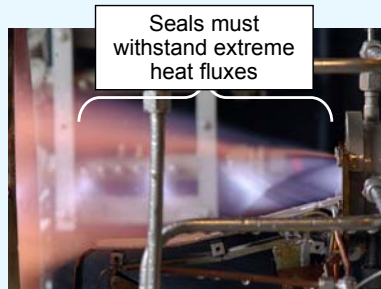
Baseline control surface seal design
