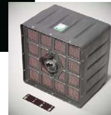
Investigation of air filters shows what material was airborne in cabin
