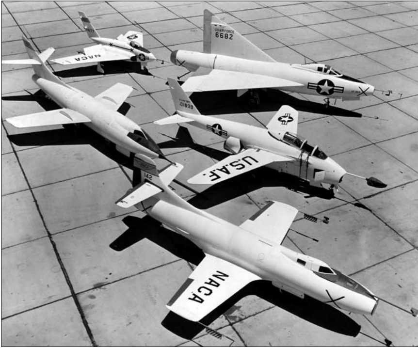
A posed group portrait of early X-planes at the NACA High-Speed Flight Station in August 1953. Clockwise from the bottom are the Douglas D55-1, Douglas D-558-2, Northrop X-4, Convair XF-92A, and Bell X-5. This group represents a wide variety of research programs, and only the D558-2 was a true high-speed airplane. (NASA)
