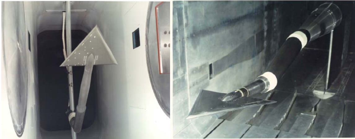
Figure 6. LTPT and NTF delta wings.
