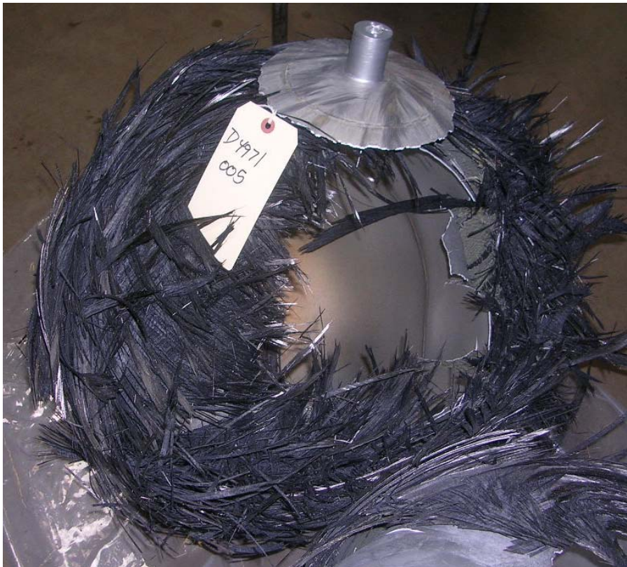
Figure 9. Cryogenic Burst Test Vessel Part No. D4971, S/N 005
