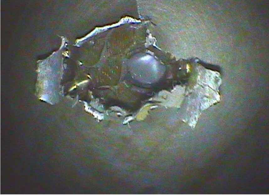
Figure 3: 12mm by 19mm hole in the rear facesheet of the radiator panel
