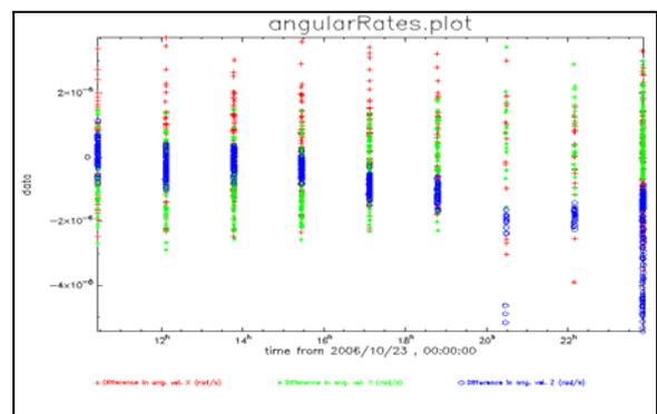
Figure 9a: Angular velocity drift daily evolution
