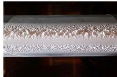
Fig. 20 Tracing and photograph of spanwise-ridge shape EG1159.
