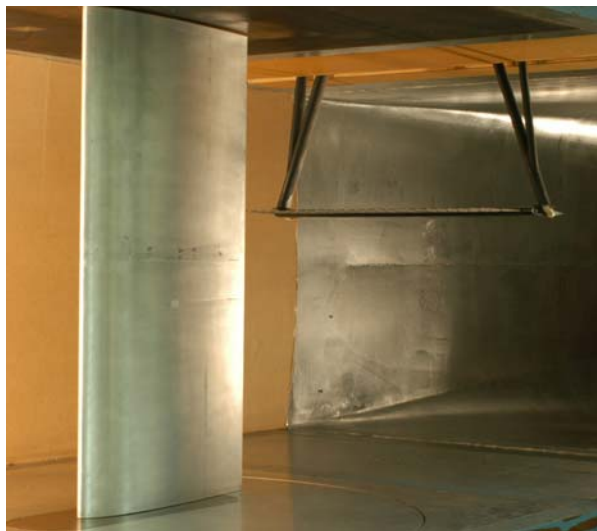
Fig. 8 Subscale NACA 23012 aerodynamic model installation in University of Illinois wind tunnel.
