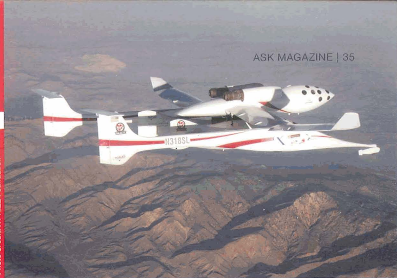
High above the Mojave desert, White Knight carries SpaceShipOne aloft for the first of its two Ansari X PRIZE-winning flights.
