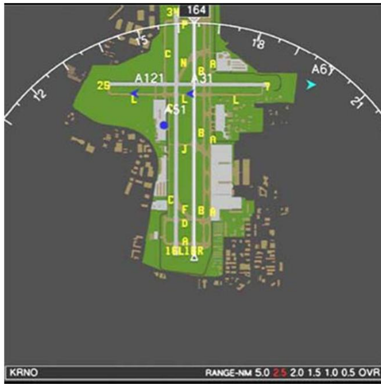
Figure 83. GA RIPS overhead view of airport surface.
