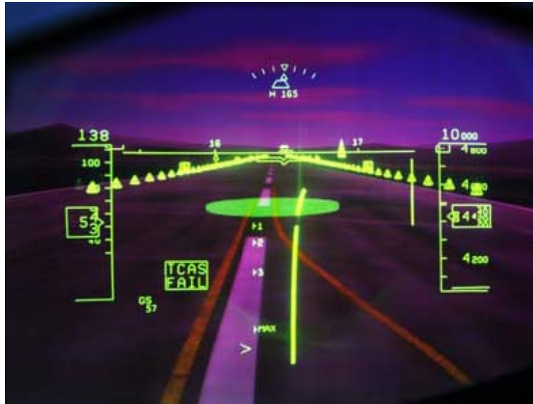
Figure 14. Illustration of RIPS HUD landing/rollout deceleration guidance format (all HUD symbology is monochrome green).
