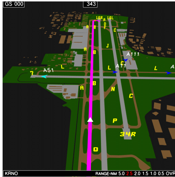
Figure 16. RIPS Electronic Moving Map (EMM).
