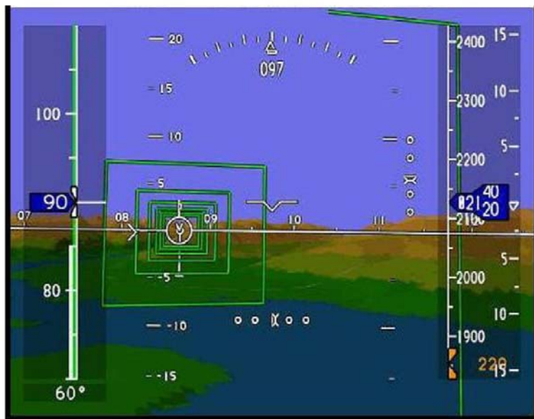
Figure 76. GA Unconnected Box Tunnel display concept.
