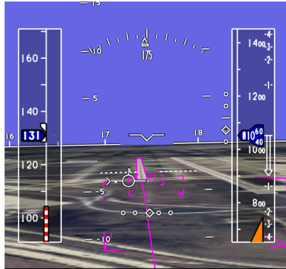
Figure 44. Image of ARINC Size-D display for 30° FOV, approximately 1.5 nm from a DFW runway.
