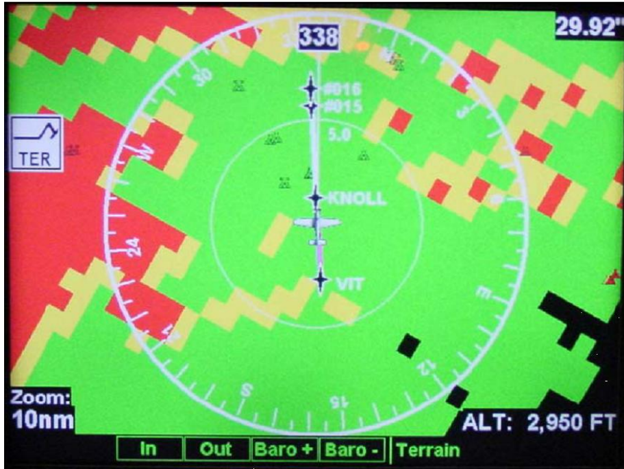
Figure 79. GA ND with TAWS implemented on an Mx-20 (on approach to ROA).
