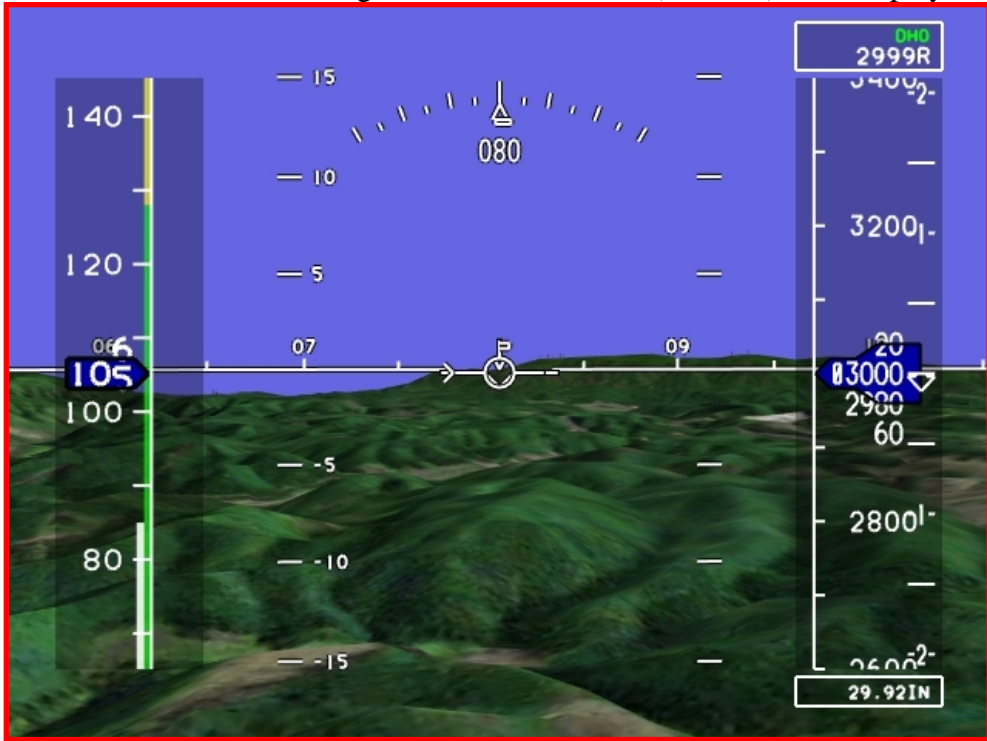
Figure 70. GA elevation based generic with a fish-net (EBGFN) SVS display concept.
