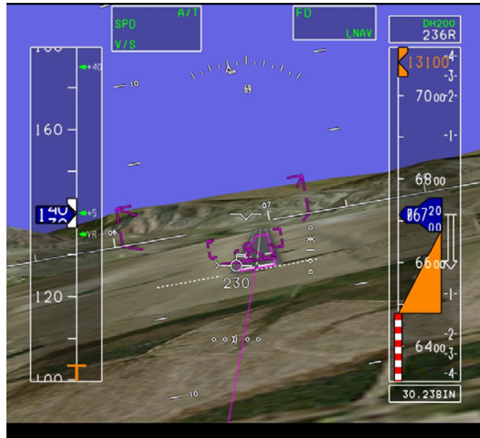
Figure 19. The wire-frame display element of the SVS PFD.
