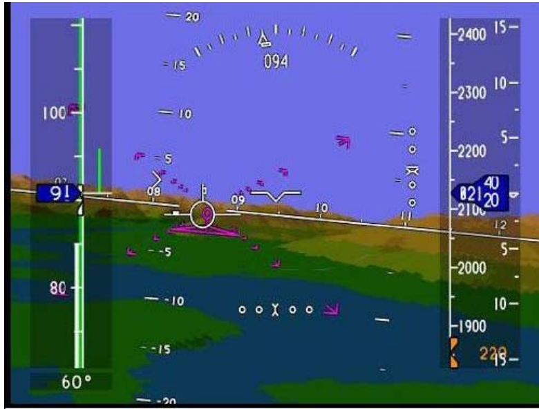
Figure 40. GA PFD with horizon line gapped about the velocity vector symbol.
