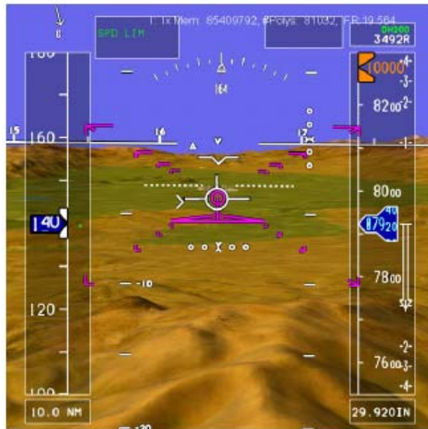
Figure 32. The HDD minimal tunnel concept used at the EGE flight trials.
