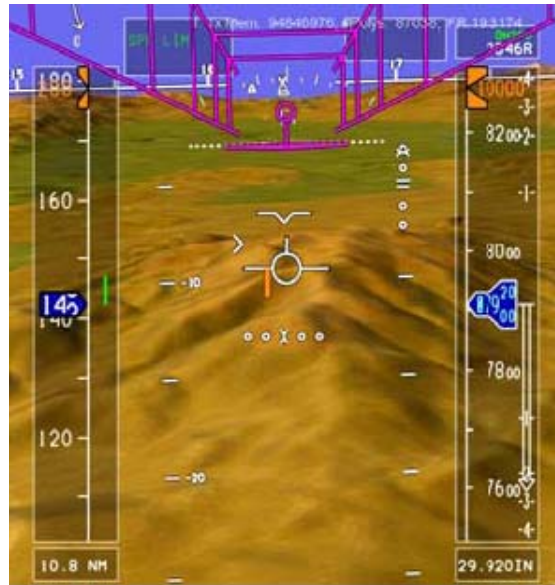
Figure 34. Outside the dynamic tunnel concept.
