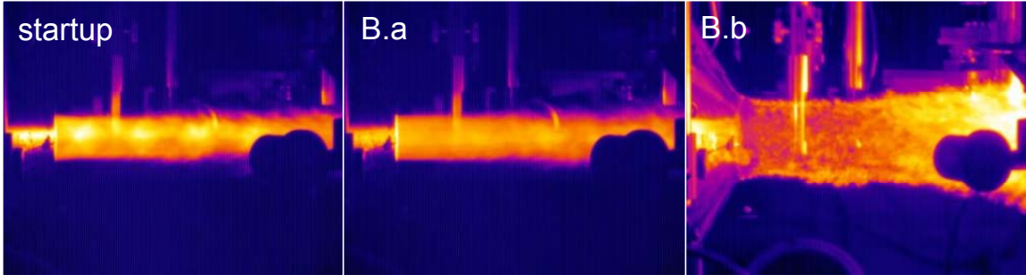
Figure 8. IR images of large scale flame during facility startup, Cases B.a ( M_h=5.5 ), and B.b ( M_h=5.5 , H_2 coflow at \phi=1 ).
