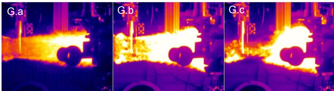
Figure 12. Cases G.a, G.b, G.c, M_f=6 and H_2 or mixed H_2-C_2H_4 coflow, showing detachment as H_2 rate is decreased.
