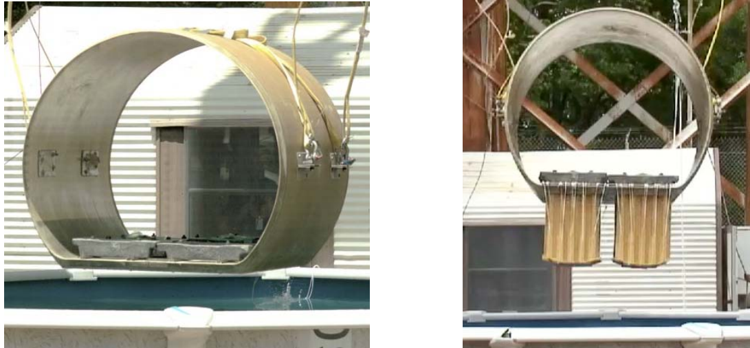
(a) Fuselage section without energy absorbers. (b) Fuselage section with energy absorbers.
