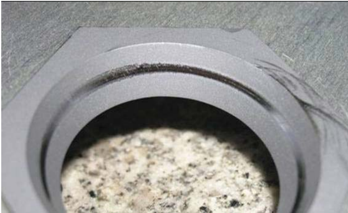
Figure 8. S/N 006 female shear tie, showing acceptable wear pattern
