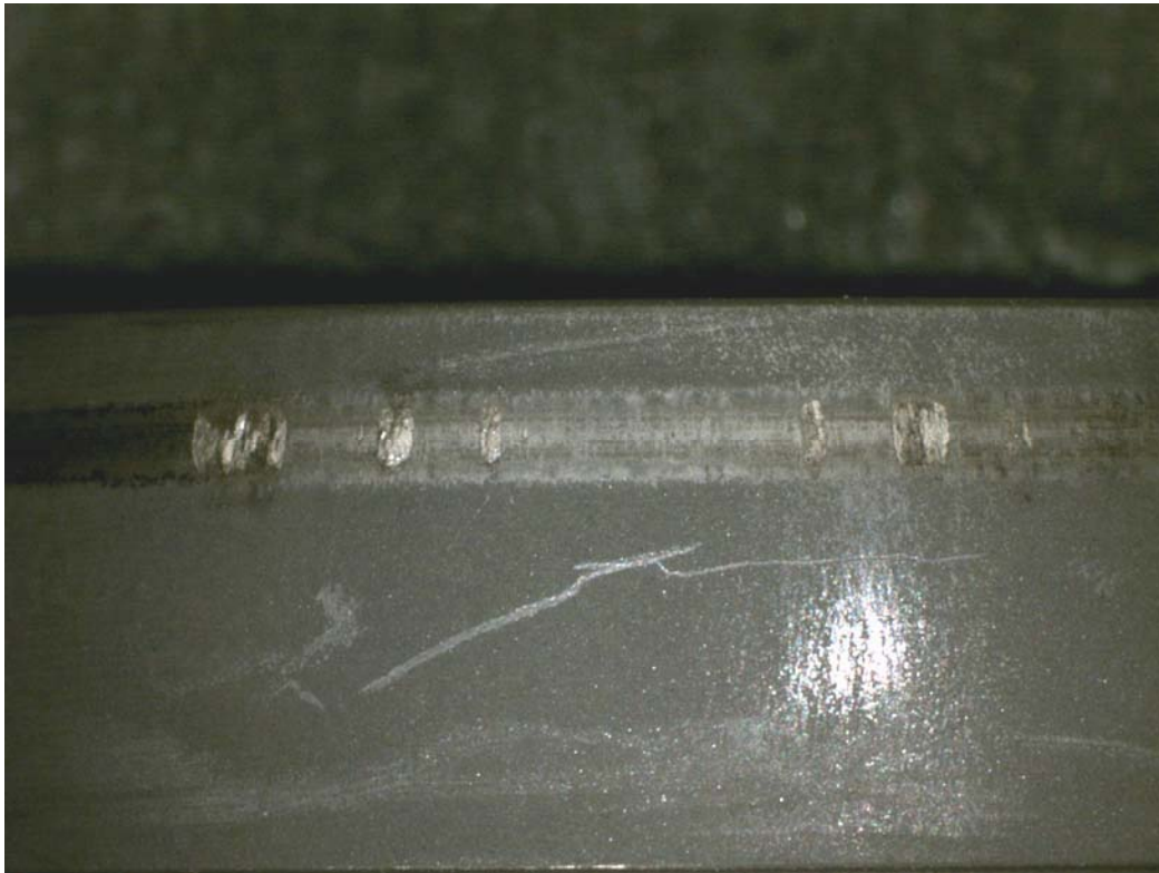
Figure 3. Photograph showing galled test specimen (unacceptable wear pattern)
