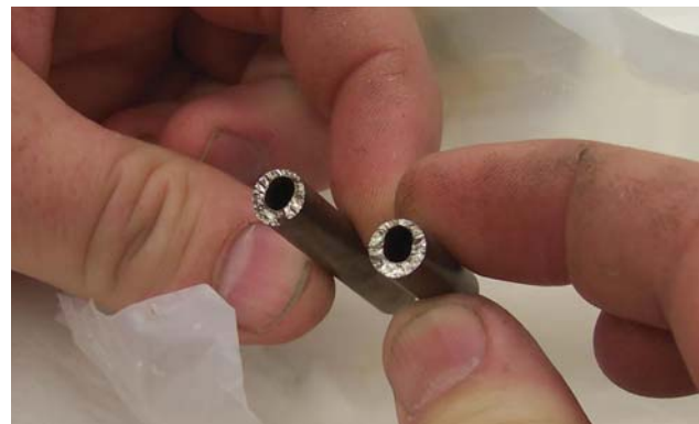
Figure 2. Terfenol-D Is Very Brittle.
