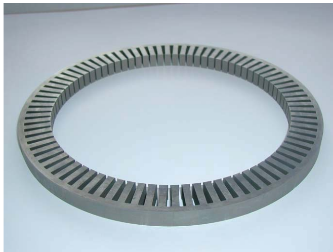
Figure 8. Thin Sheet Stacking with Structural Bonding
