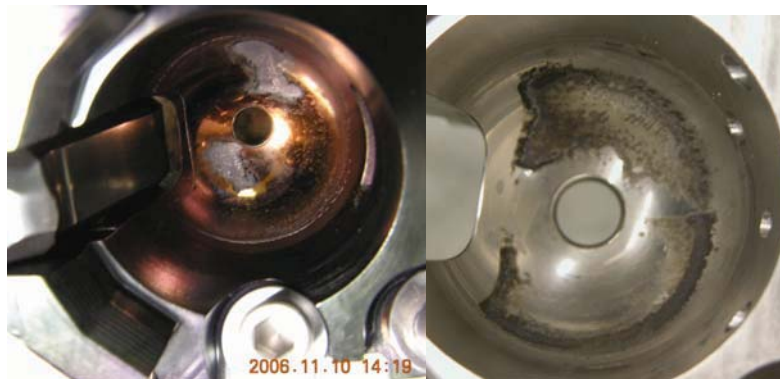
Figure 12. Right: DLN coating failure due to lack of pre-load. Left: Bare metal case
