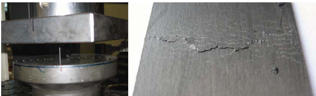
Figure 9. Test set-up and destroyed compression sample
