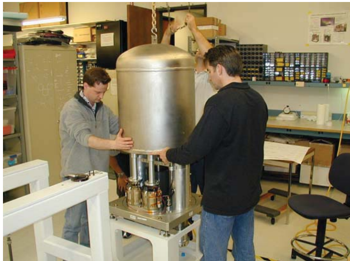
Figure 6 Trial-fitting of vacuum housing onto suspension device.
