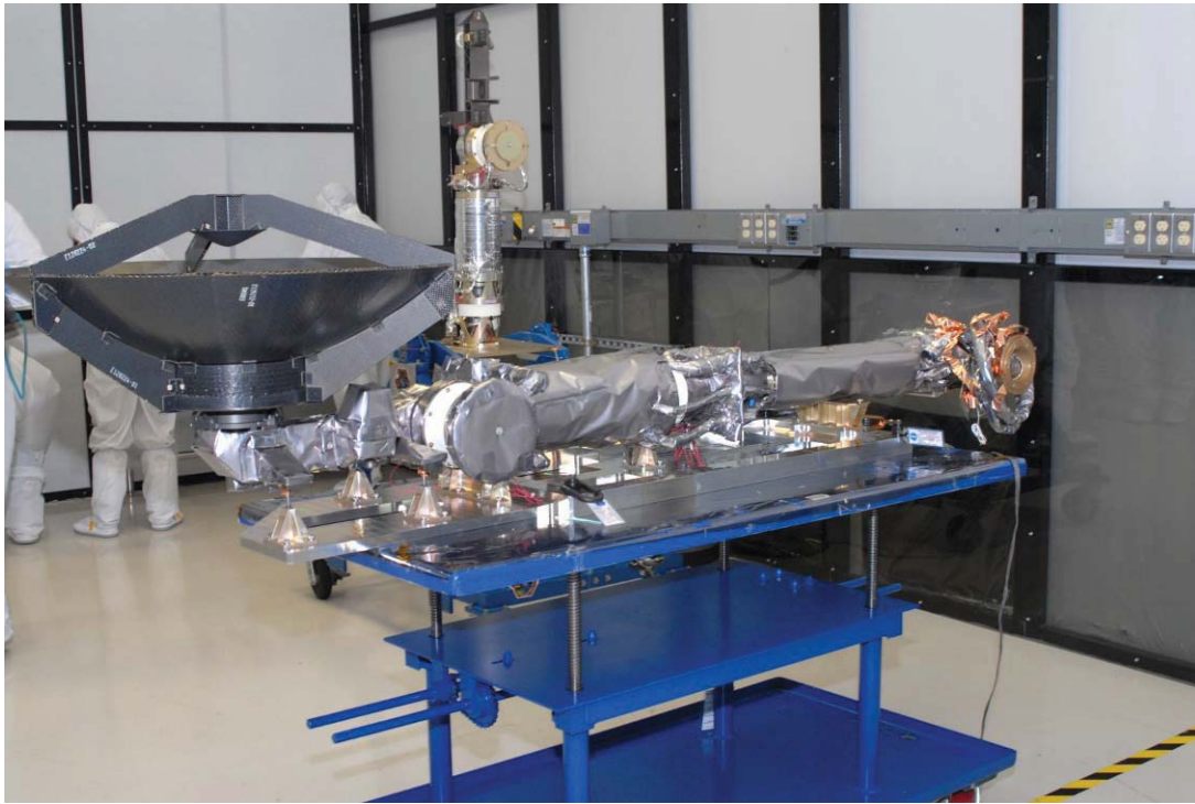
Figure 8. SDO Gimbal Mated to Deploy Boom and High Gain Antenna, with MLI installed Second Unit Shown Vertical in Background
