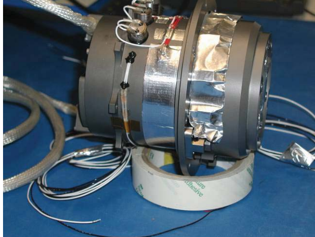
Figure 3. Rotary Actuator Shown During Thermal Hardware Application
