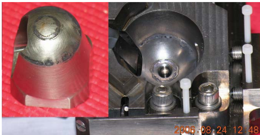
Figure 10. Damage of B 4 C observed due to qualification level testing
