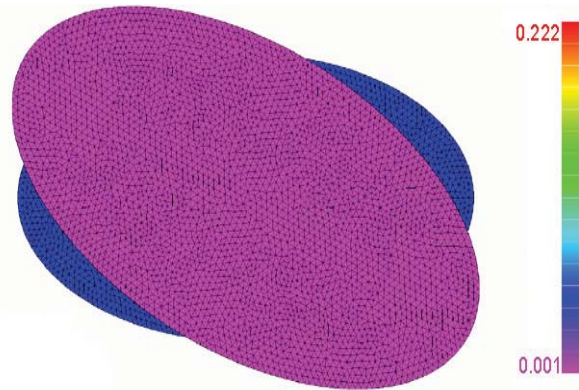
Figure 4. Mirror Mode 1, Torsional about Z-Axis, 270 Hz
