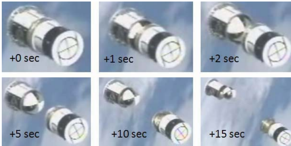
Figure 8. Actual On-Orbit ICU Separation Event
