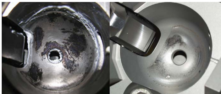
Figure 13 L: Braycote to Ti6Al4V interface R: Tiodize and MoS 2 after RV and T-vac Testing
