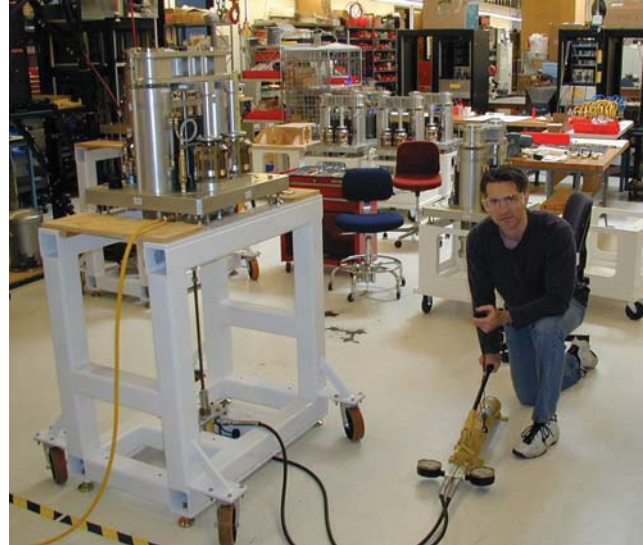
Figure 17 Setup for proof load test of suspension device
