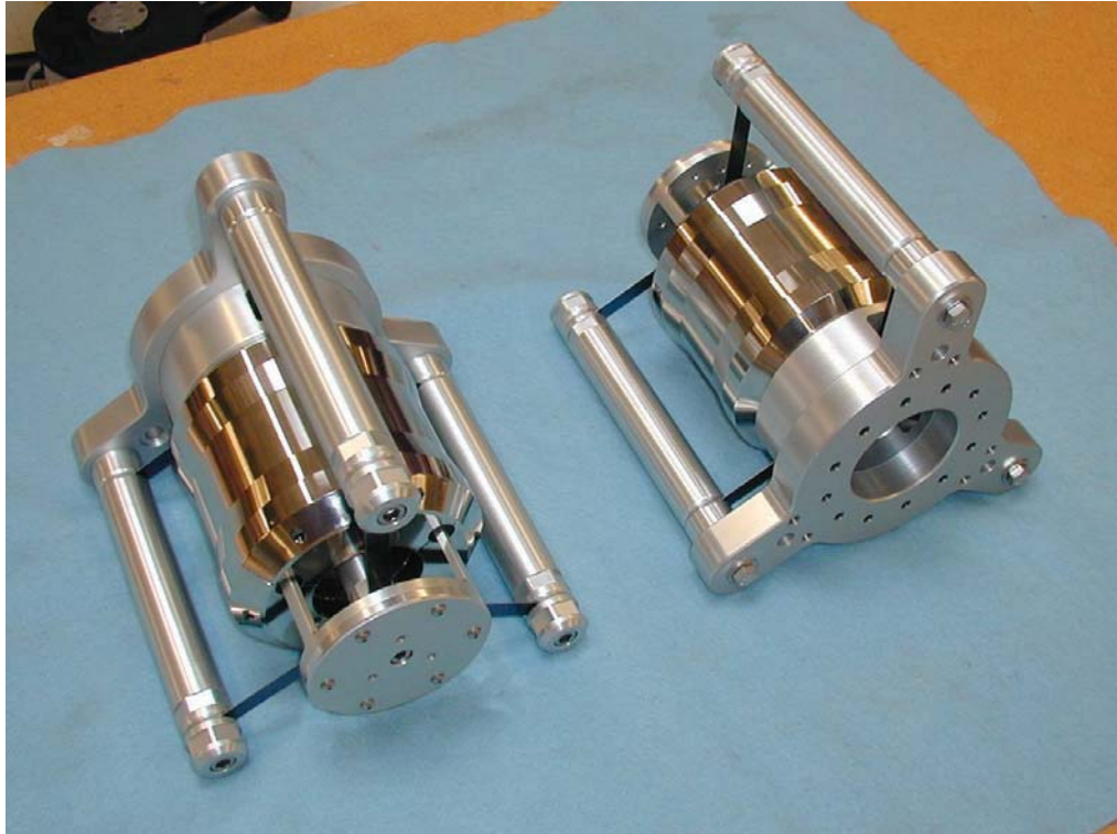
Figure 9 Passive magnetic dampers for payload pendulum modes
