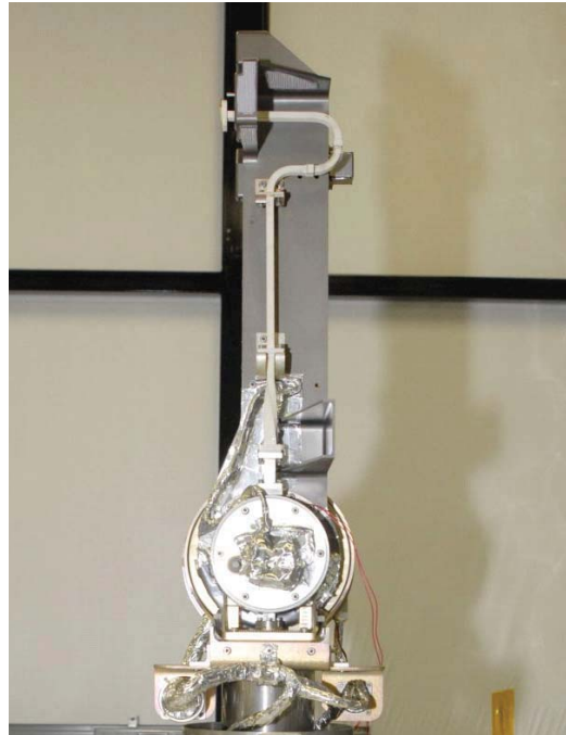
Figure 7. Waveguide Resolution - Elevation Waveguide with “P-Trap” section
