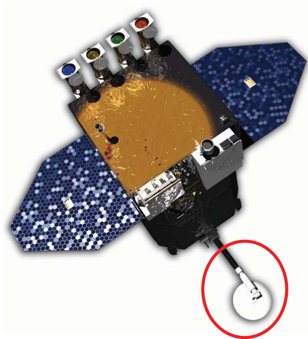
Figure 1. Solar Dynamics Observatory with One of Two High-Gain Antennas and Gimbals Circled
