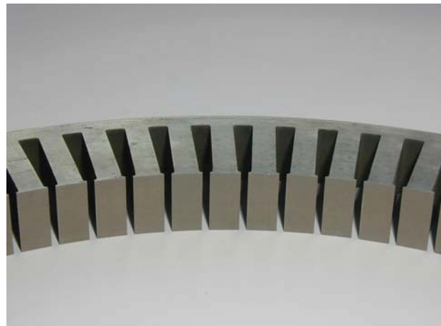
Figure 2. Thin sheet stacking with notches
