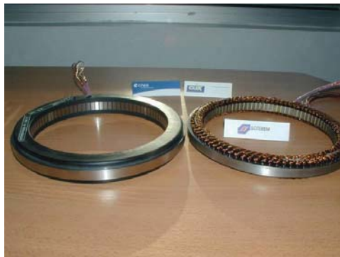
Figure 7. Existing Referenced Stator and the Structurally Bonded Stack
