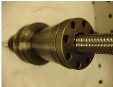
Figure 9: Ballnut bolted to Drive Link
