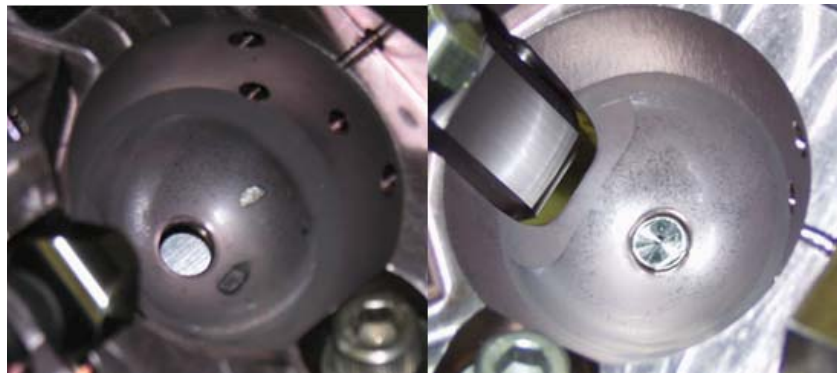
Figure 16 L: First TiCN-MoS 2 try. R: Successful TiCN-MoS 2 qual testing
