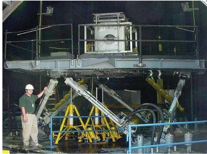
Figure 7: 6-DOF testing facilities at MSFC
