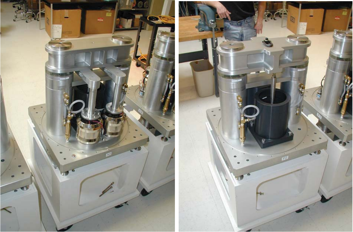
Figure 5 Suspension devices. Type A, augmented (left), Type P, passive only (right).
