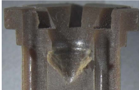
Figure 11. Split Spool Deformation
