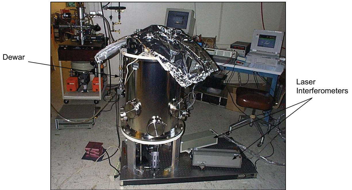
Dewar with Laser Interferometers (Quad-Cell Autocollimators not shown)
