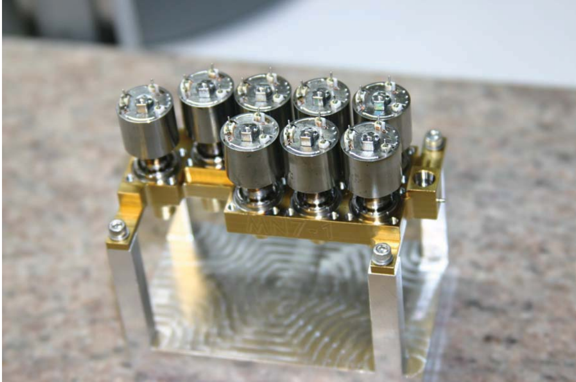
Figure 7 - Flight Microvalves Welded into a Flight Manifold
