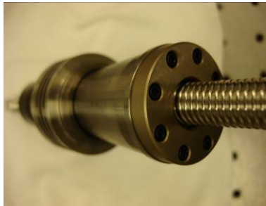
Figure 9: Ballnut bolted to Drive Link
