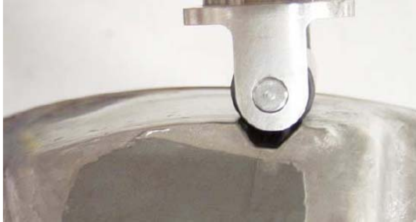
Figure 5: Roller locked in the detent groove when the valve is in the open position
