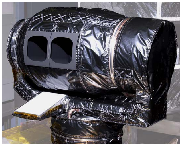
Figure 2: The Completed MCS Instrument
