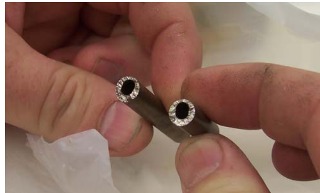
Figure 2. Terfenol-D Is Very Brittle.
