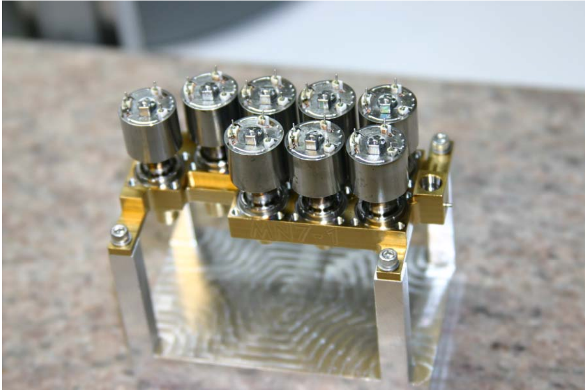
Figure 7 - Flight Microvalves Welded into a Flight Manifold
