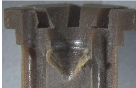
Figure 11. Split Spool Deformation
