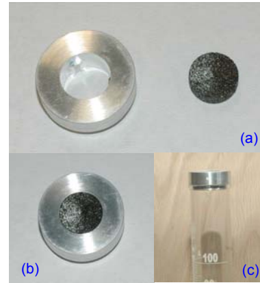
Fig. 6. Foam liquid flow rate test apparatus; (a) aluminum holder and Poco foam sample, (b) Poco foam inside aluminum holder, (c) Poco foam and holder at top of graduated cylinder
