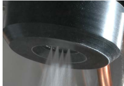
Fig. 4. Spray Manifold Close-up of 2x2 Nozzle Array
