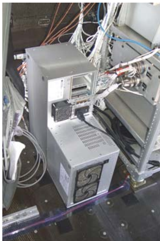
Fig. 3-13 Unit PXI-1010 at its final location behind the pilot seat.
