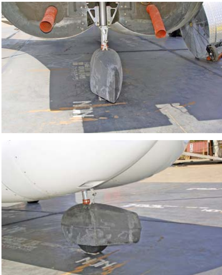
Fig. 4-3 Configuration with deployed faired nose wheel for in ground effect tests.
