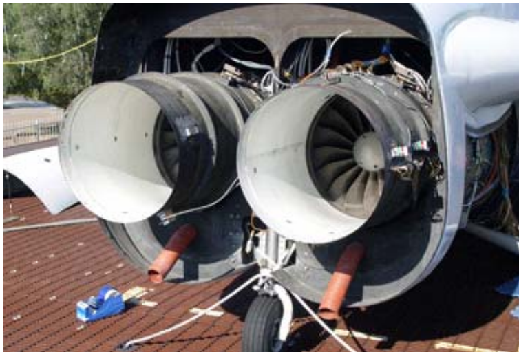
Fig. 3-9 View of instrumented inlets with front cowling removed.
