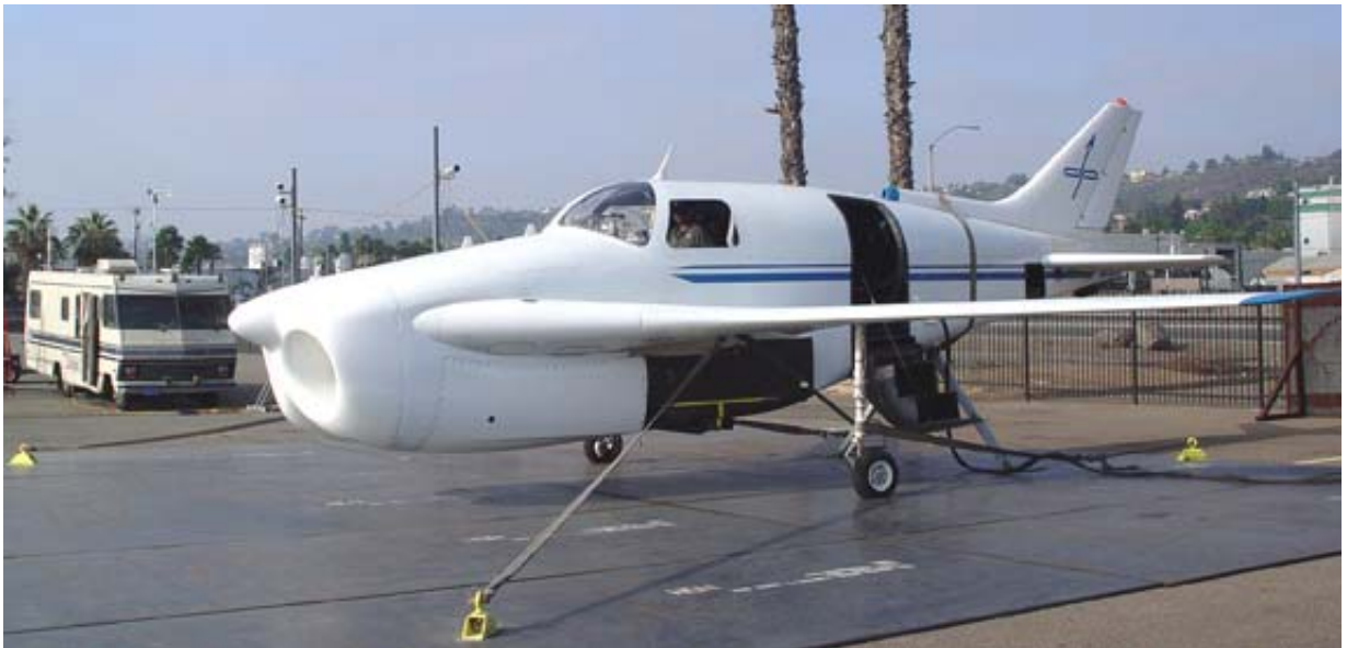
Fig. 4-4 Configuration with removed nose wheel for in ground effect tests.
