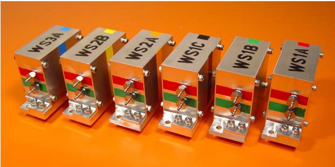
Fig. 2-6 Assembled wall pressure modules (view from 'pneumatic end').
