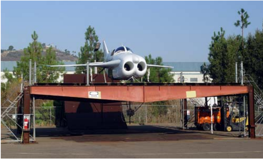
Fig. 1-1 DP-1C aircraft on an elevated platform for OGE testing.
