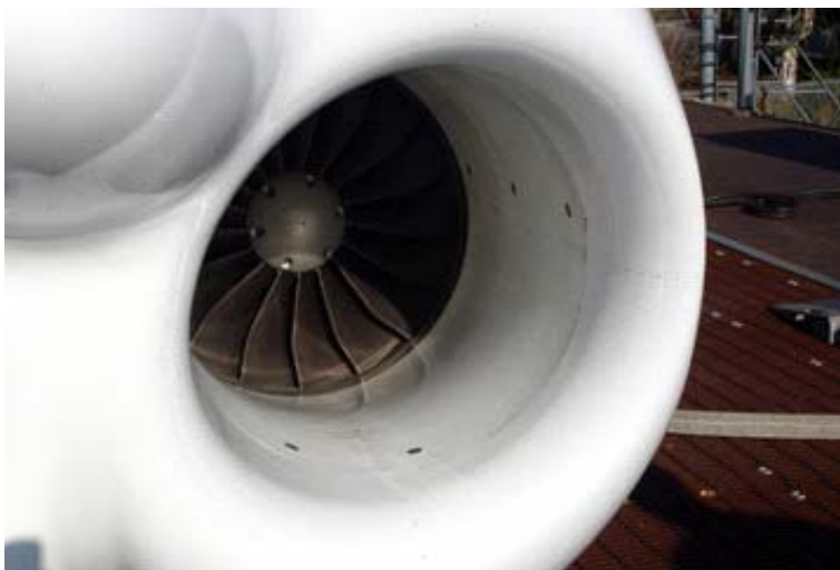
Fig. 3-10 Fully instrumented left engine inlet.
