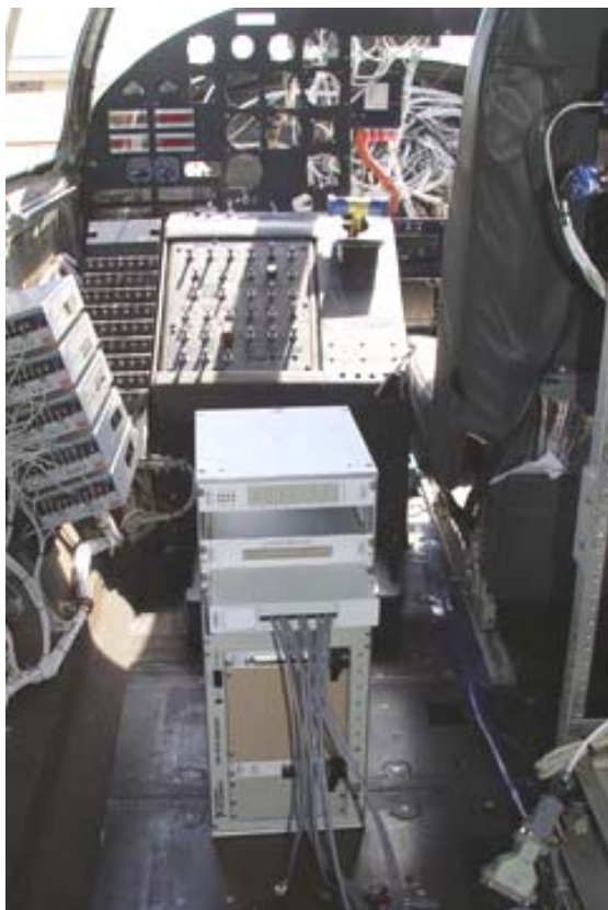
Fig. 3-12 Data acquisition unit PXI-1010 on board during shake down tests.
