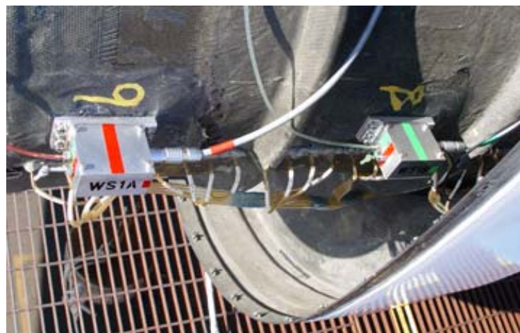
Fig. 3-7 Pressure modules plugged into ports L030 and L035.
