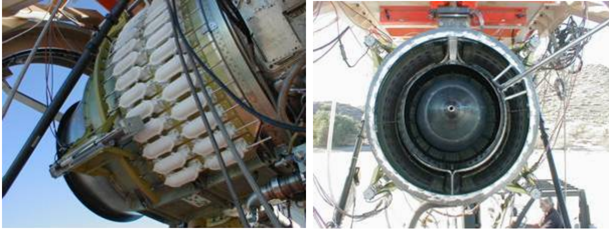
Figure 662. Exhaust Rotating Rake Test Configuration 73, Acoustically Treated Duct With HQ Tube Balls In Forward Position, Was Completed On March 8, 2007.
