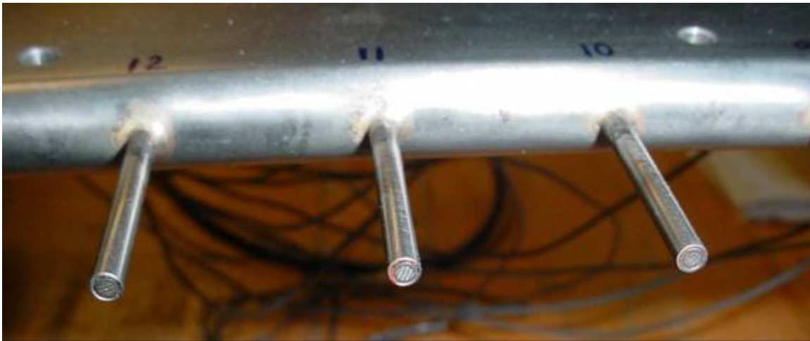
Figure 617. The Functionality Of The Transducers In The Inlet Rake Arm Were Evaluated.
