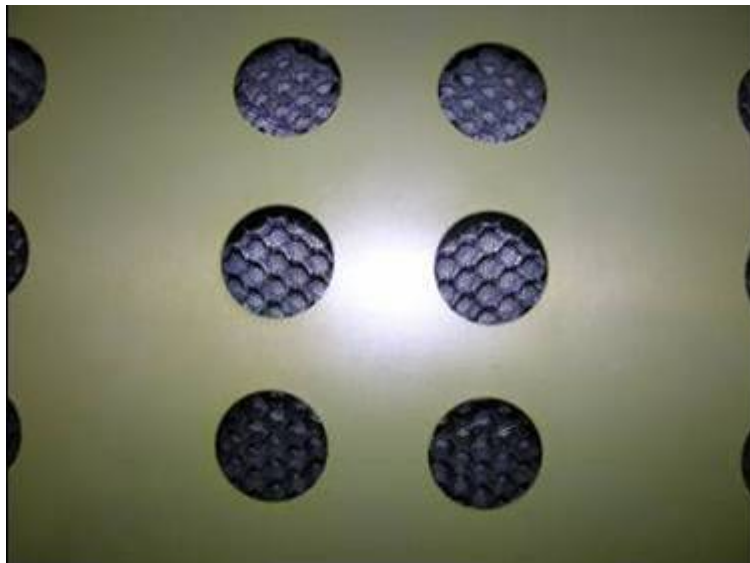
Figure 36. This Close-Up View Of The Backing Skin Shows The Honeycomb Core And The Porous Facesheet Of The Passive Liner.
