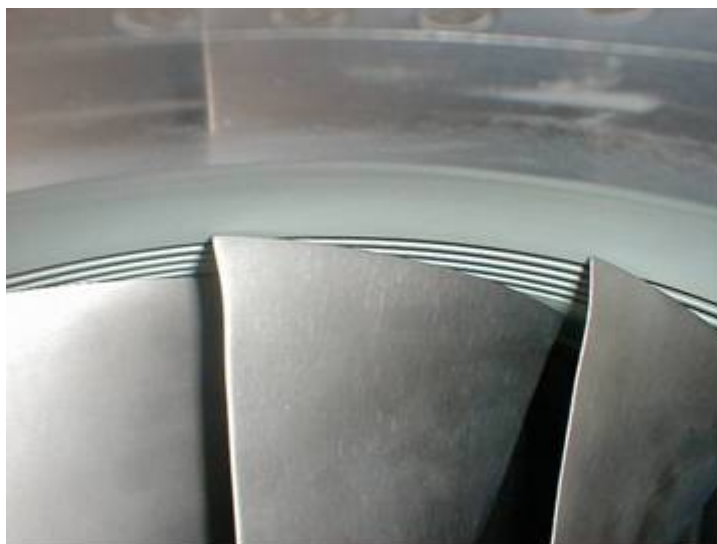
Figure 162. Close-Up View Of The Fan Tip Casing Treatment For The Engine Scale Quiet High Speed Fan II Installed On The TECH7000 Engine.
