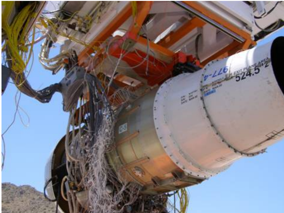
Figure 553. Instrumented Exhaust By-Pass Duct On The TECH977.
