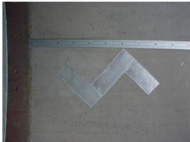
Figure 640. Configuration 45: Irregular Patch, Close To Fan, At Current Inlet Repair Limits.
