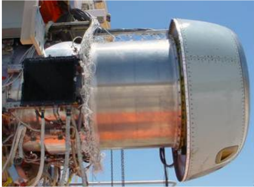
Figure 527. The Instrumented Spool Piece For The Inlet Phase Array Extends The Inlet 36 Inches Forward Of The Baseline Position.
