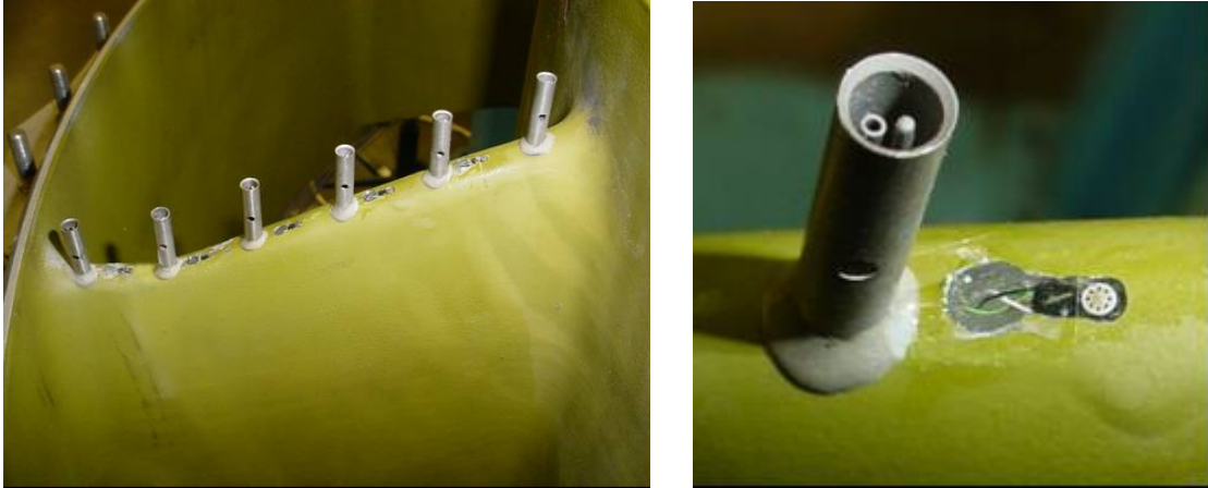
Figure 282. Five Kulites Were Flush-Mounted Along The Leading Edge Of The Front Frame, Positioned In Between The Total Pressure Probes.
