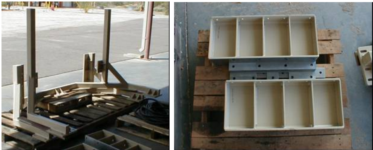
Figure 318. Fabrication Was Completed For The Modified Support Frame, The Spacer Brackets, And Mounting Brackets.
