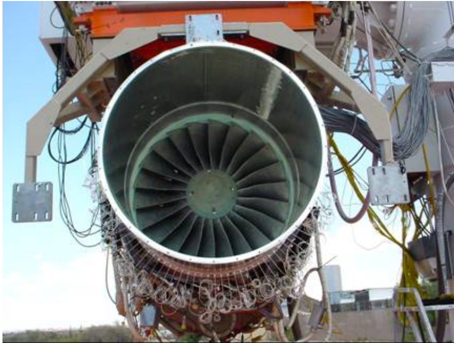
Figure 526. Instrumented Inlet Spool Piece With 119 Total Kulites, 90 Around The Circumference And 29 Along An Axial Line Near Top Dead Center.
