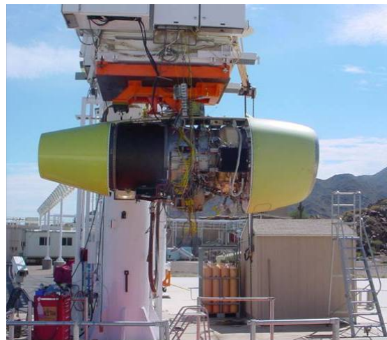
Figure 160. The TECH977 Engine Installed In The Honeywell Acoustic Stand.
