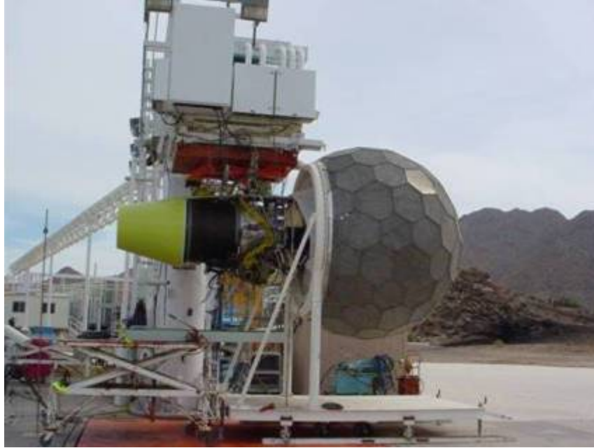
(a) TECH977 turbofan engine mounted on testing rig with ICD (Aft Barrier Not Shown).
