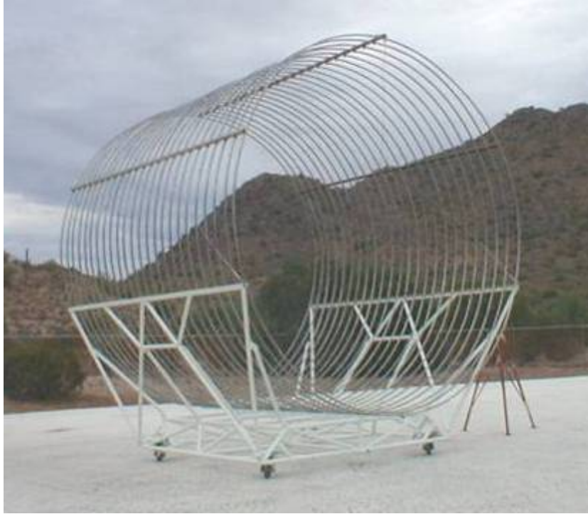
Figure 574. The Cage Array Structure At The San Tan Test Facility.
