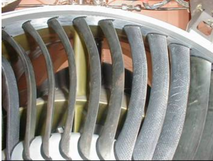
Figure 163. Close-Up View Of The Stator-Strut Alignment OB The Quiet High Speed Fan II Installed In The TECH7000 Engine.
