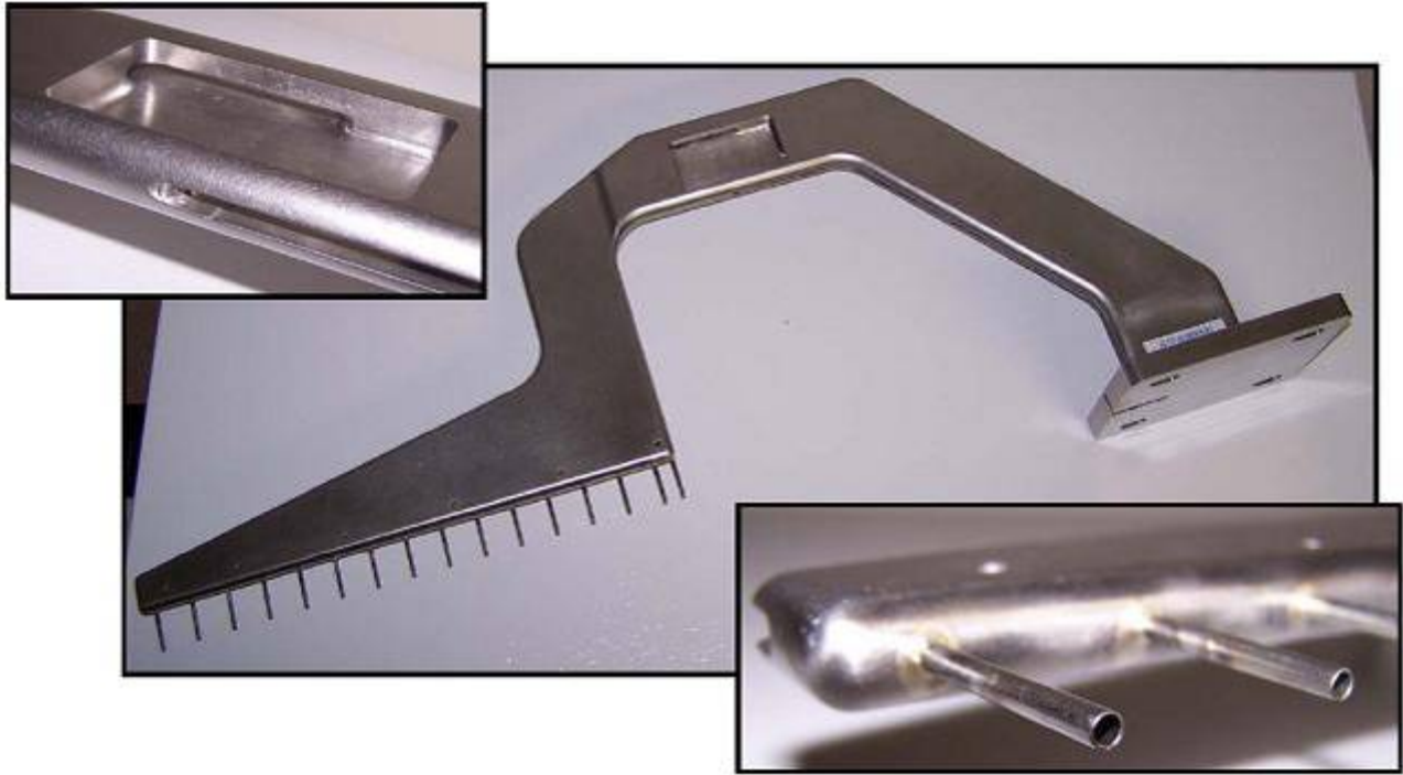
Figure 316. Transducer Tubes Were Brazed Into The Rotating Inlet Rake Arm.
