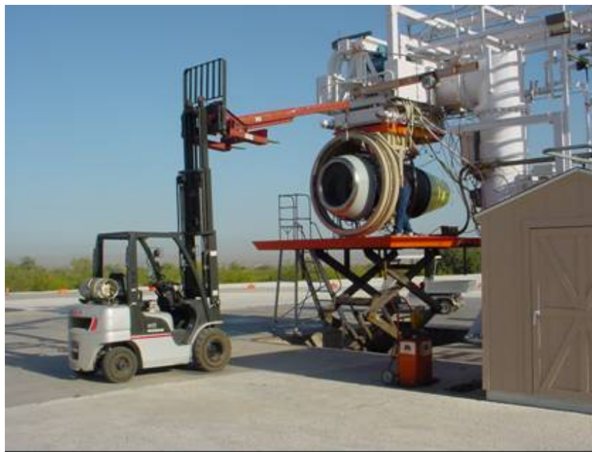
Figure 611. A Forklift Positions The Rotating Rake On The Inlet Of The TECH977 Engine.
