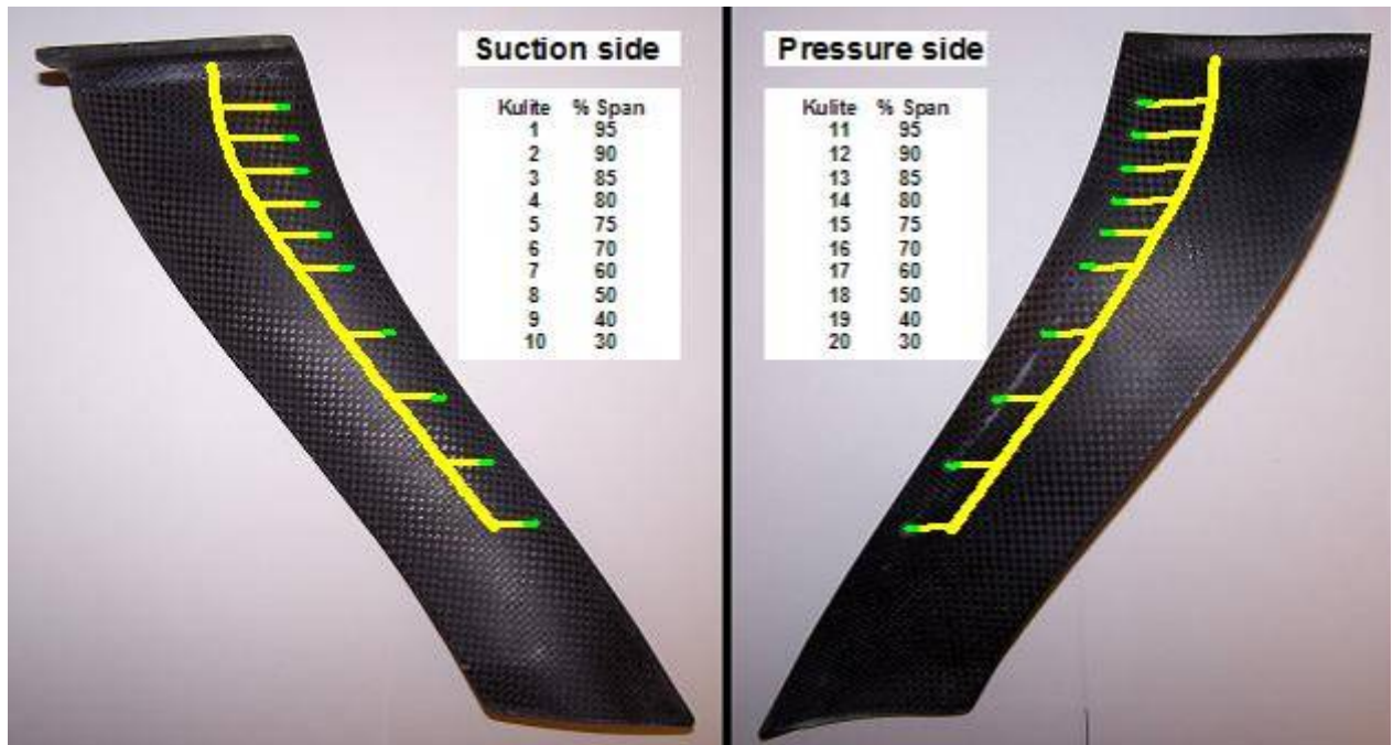
Figure 289. Locations Of The 20 Absolute Pressure Transducers For The Vane Dynamic Pressure Measurements Were Finalized.
