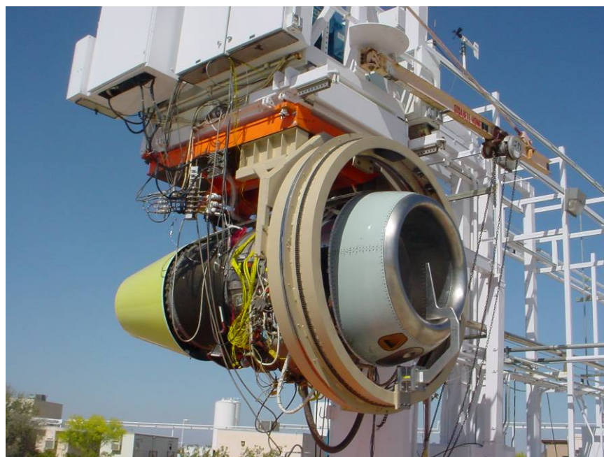
Figure 612. The Rotating Rake Was Installed On The TECH977 Engine.
