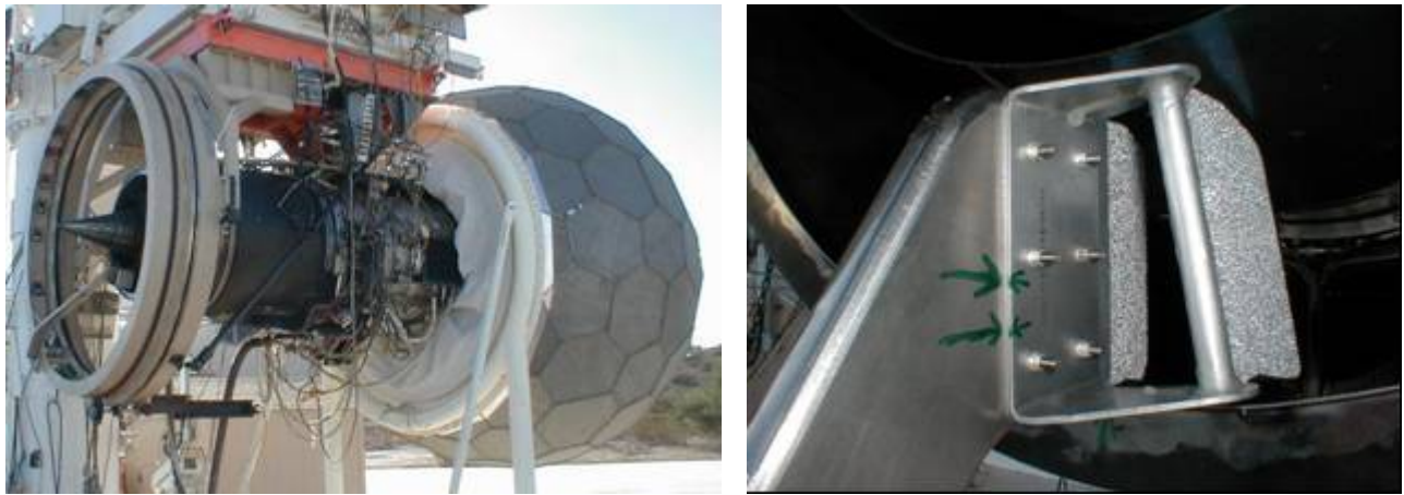
Figure 657. The Rotating Exhaust Rake System Was Installed In The Aft Position [Left] And The Exhaust Rake Was Aligned Inside The Bypass Flowpath [Right].
