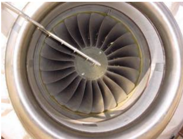
Figure 641. Configuration 46: Square Patch, Close To Fan, At Twice Current Inlet Repair Limits.
