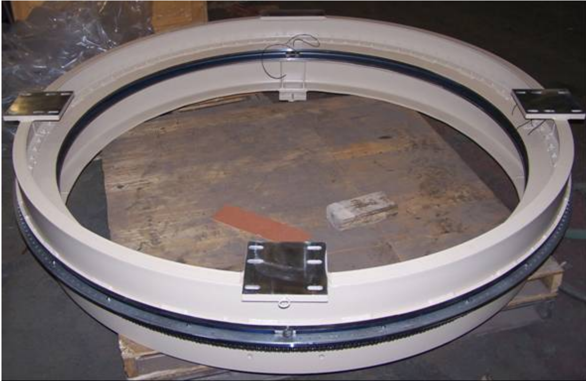
Figure 315. Major Mechanical Assembly Of The Stationary Ring And Rotating Ring Was Completed, As Shown In This Assembled View.
