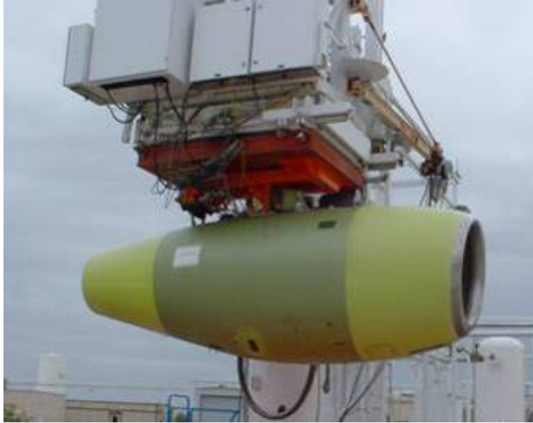
Figure 388. Noise Testing Was Conducted On The TECH977 With The Cowl Doors Installed.
