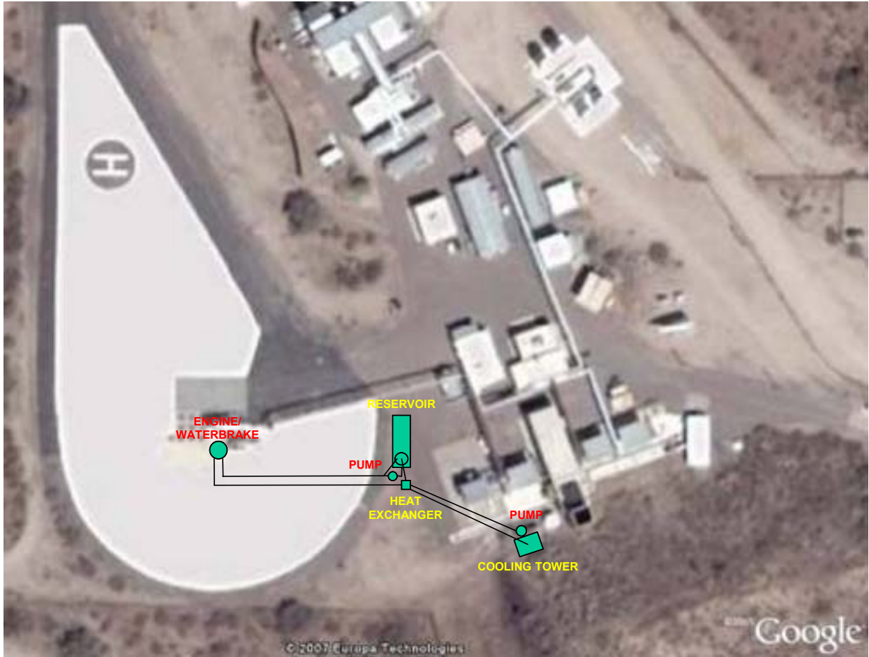
Figure 485. Run Without Fan Water Cooling Layout.
