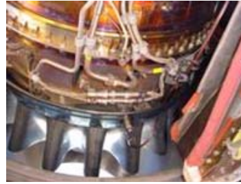
High-temperature sensors with air cooling at turbine exit
