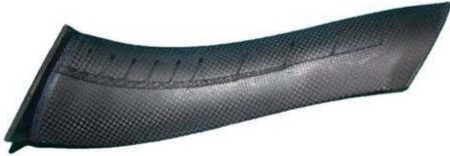
Figure 290. View Of The Vane Fabricated By Using A Rotary Hand Drill To Create Recesses For The Instrumentation And Wires.
