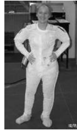
Nylon Spandex/SWNT Fabric for Spacesuits
