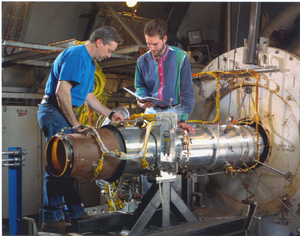
Figure 3–5 FJX-2 Installation into PSL Altitude Facility
