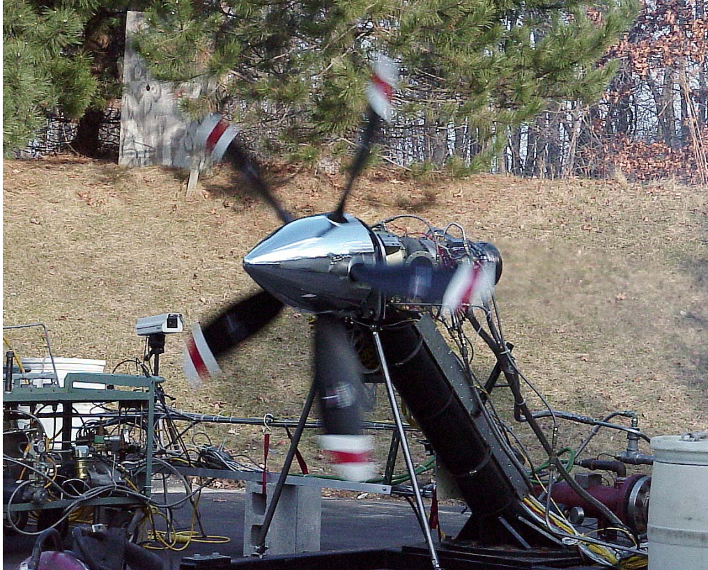
Figure 4-2 TSX-2 and McCauley Propeller in Test at OTF
