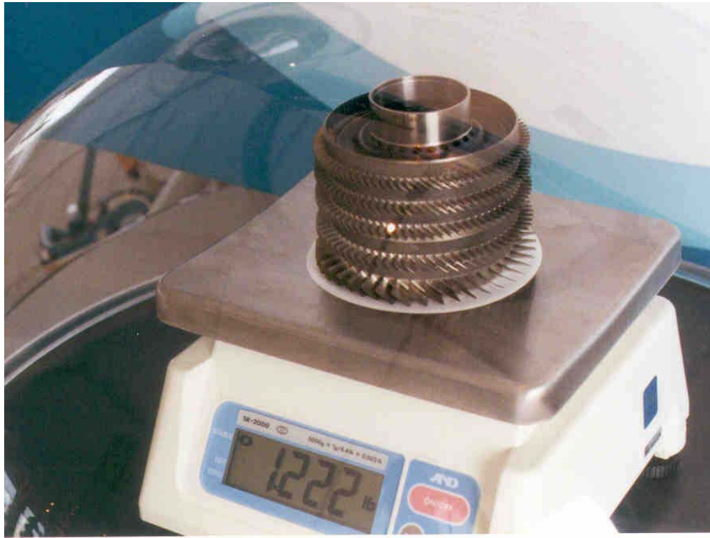
Figure 3-1 High Pressure Compressor Rotor
