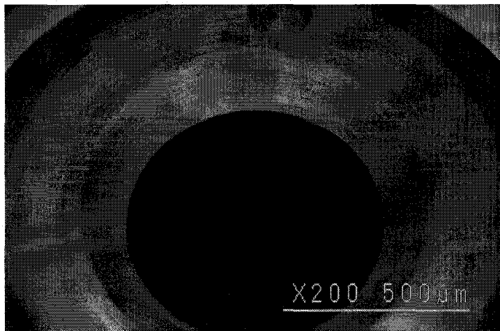
Figure 11 Crack can be seen through the compatibility testing mark and from the inner to outer diameters
