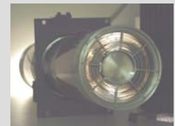
MSFC x-ray module with 12 nested mirrors
