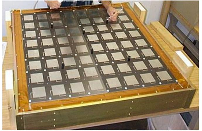
Fig. 2 Dual-polarization micro-strip patch antenna
