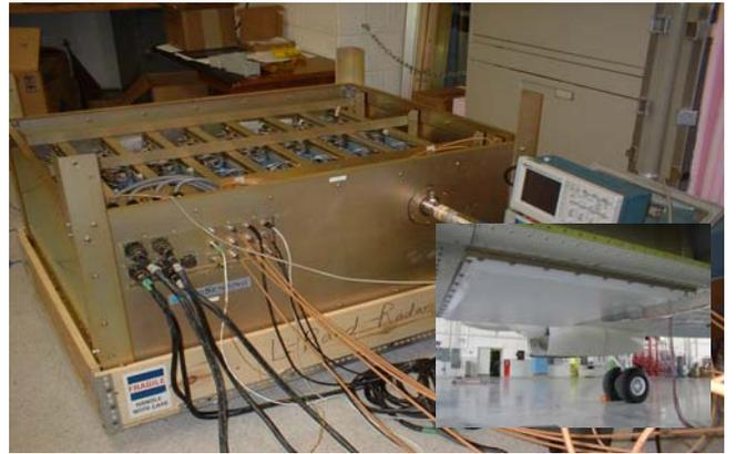
Fig 3 Radar assembly in laboratory and mounted on P3 aircraft (inset).
